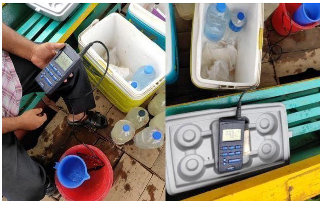
Figure 3.5: Measuring Dissolved Oxygen of the river water at a selected location.
