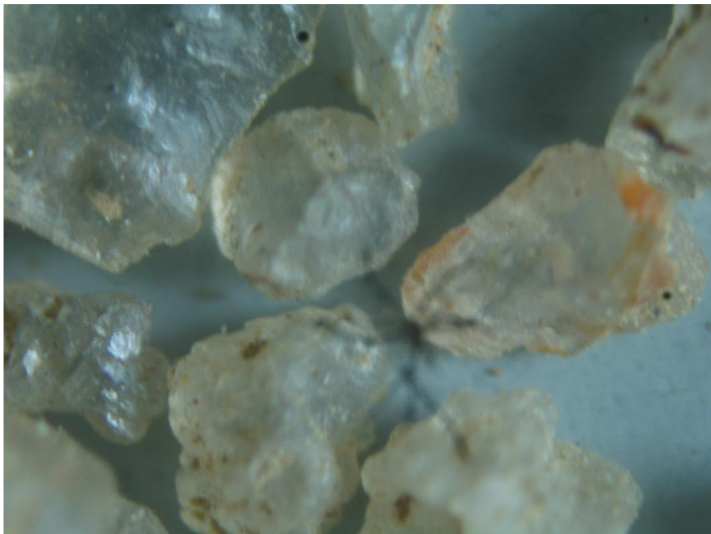
Fig. 3.8: Scanning electro microscopic view sand having mean diameter is 0.35 mm
