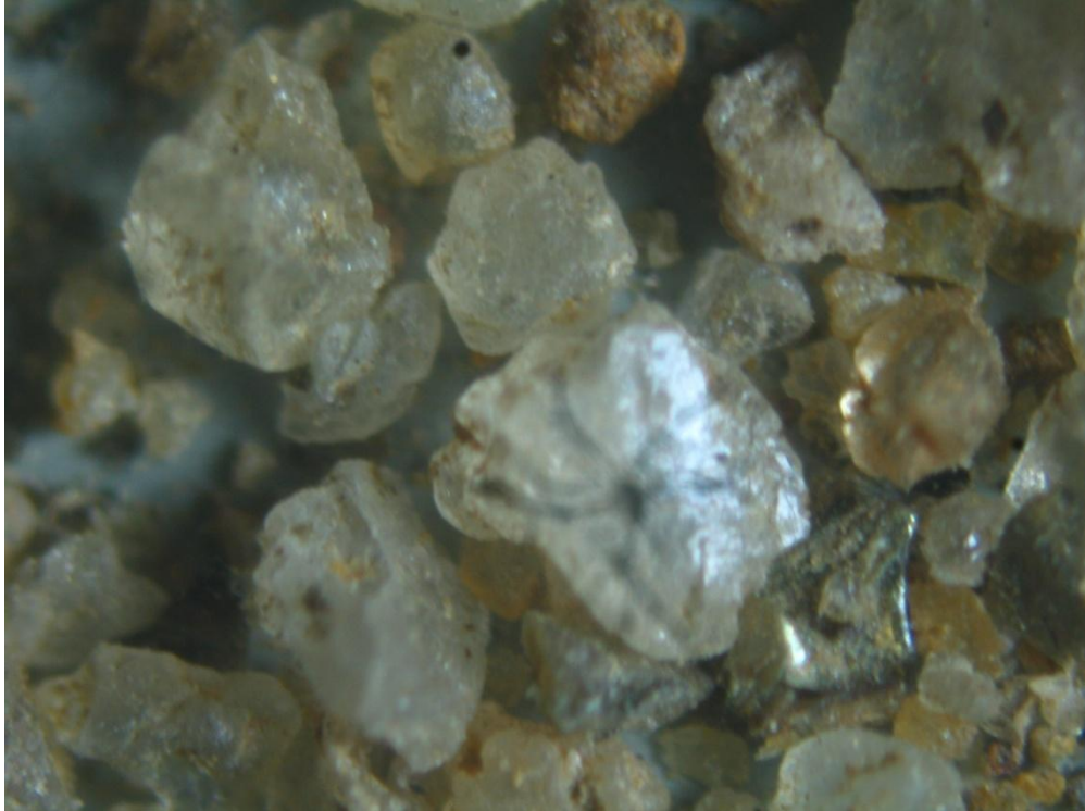
Fig. 3.7: Scanning electro microscopic view sand having mean diameter is 0.70 mm
