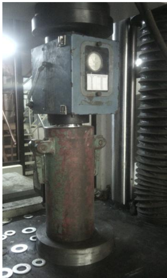
Fig. 3.16: Hydraulic jack calibration by using load column (Capacity= 500 kN) (Model No. 1052-12-108)
