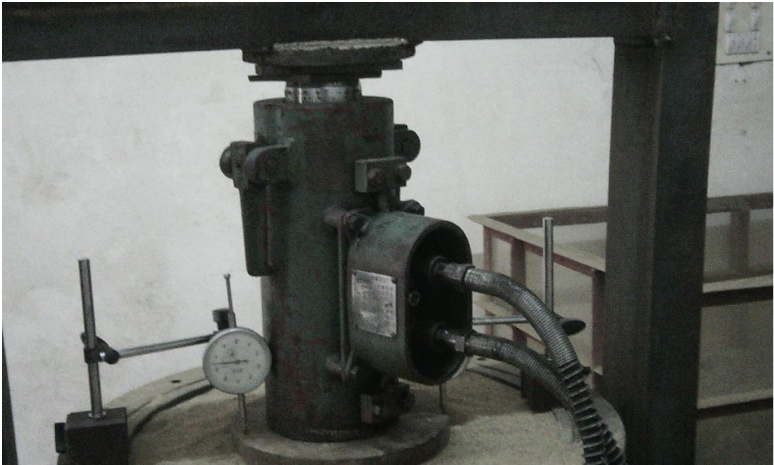
Fig. 3.25b: Load column frame with hydraulic jack at loading condition
