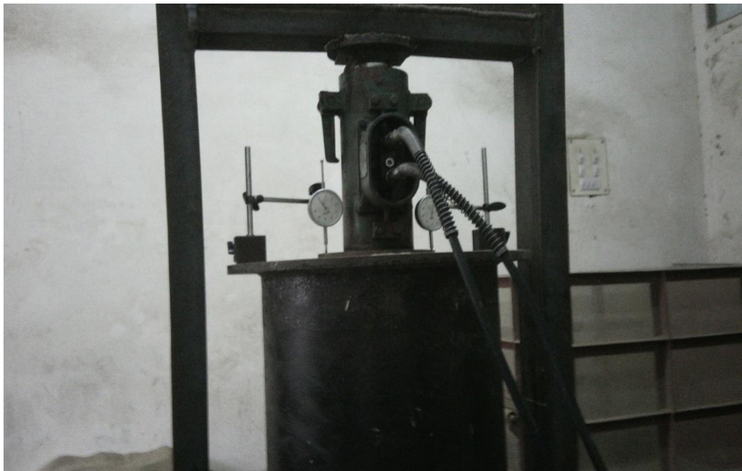
Fig. 3.25a: Load column frame with hydraulic jack at loading condition
