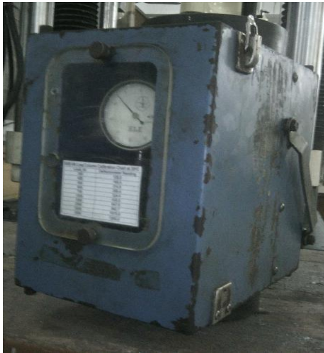
Fig. 3.15: Load column (Capacity=500 kN) (Model No. 1052-12-1085)
