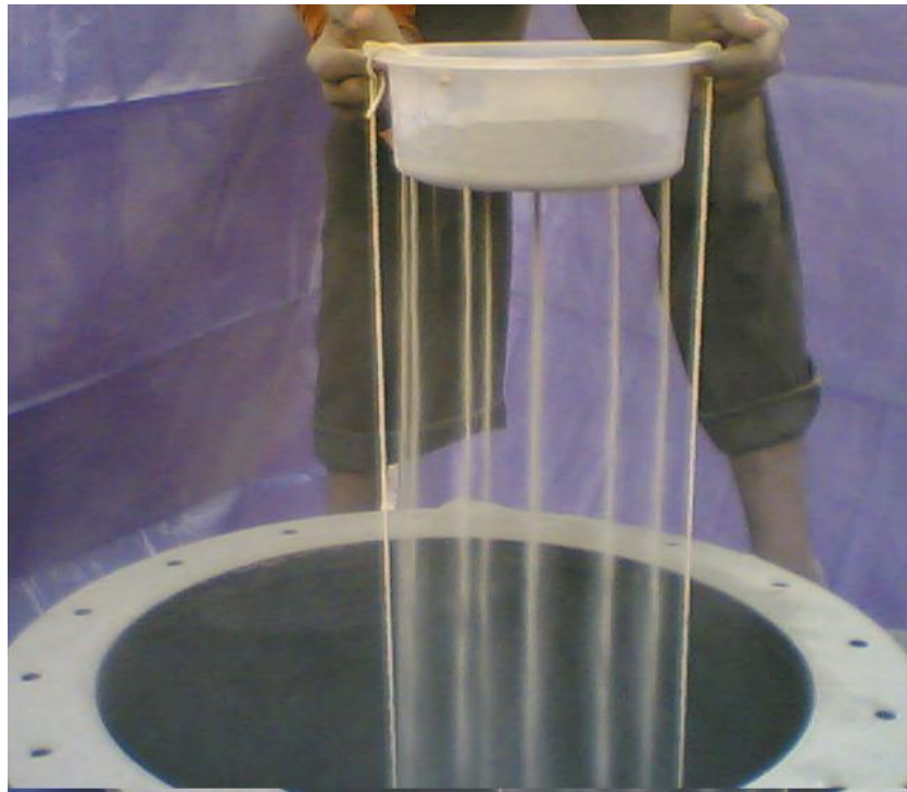
Fig. 3.9: Dry deposition into calibration chamber from discharging bowl maintaining a constant height of fall (Azad, A.K., 2008)
