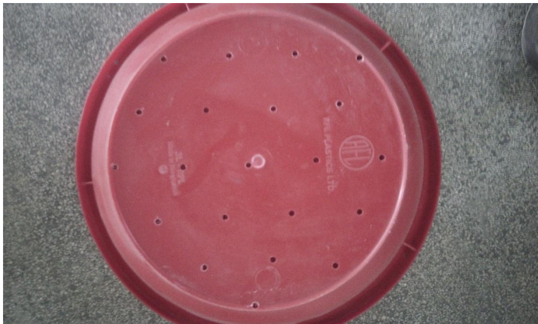
Fig. 3.2: Sand discharge bowl with 3.5mm diameter holes
