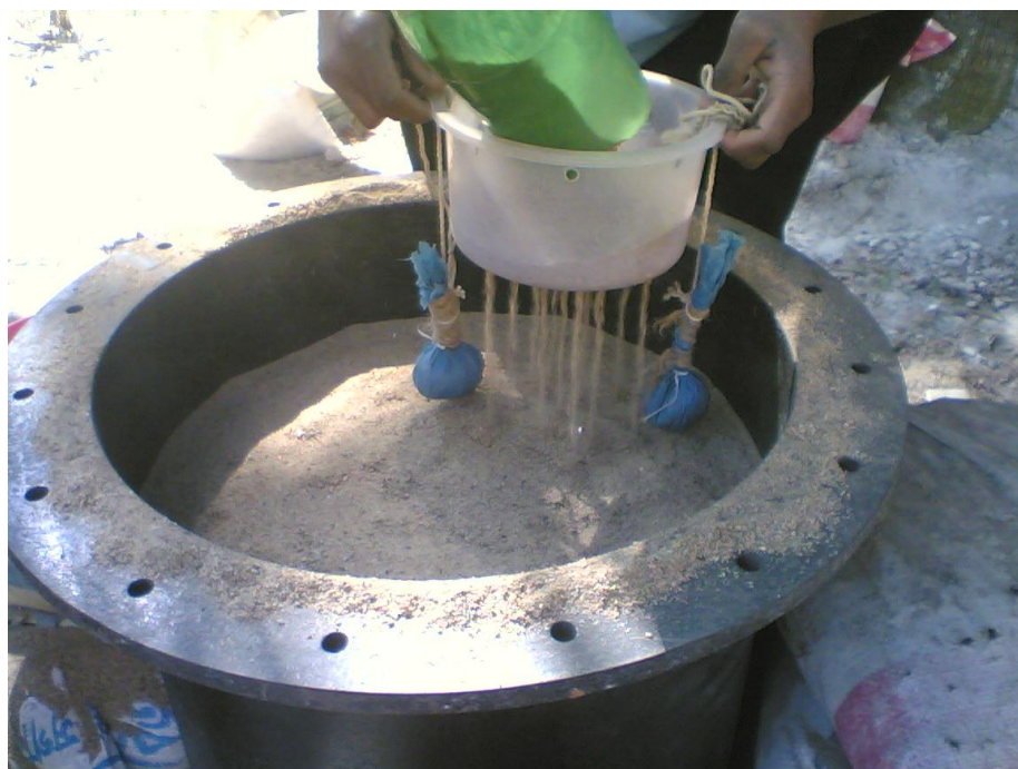
Fig. 3.10: Filling of calibration chamber in progress (Azad, A.K., 2008)
