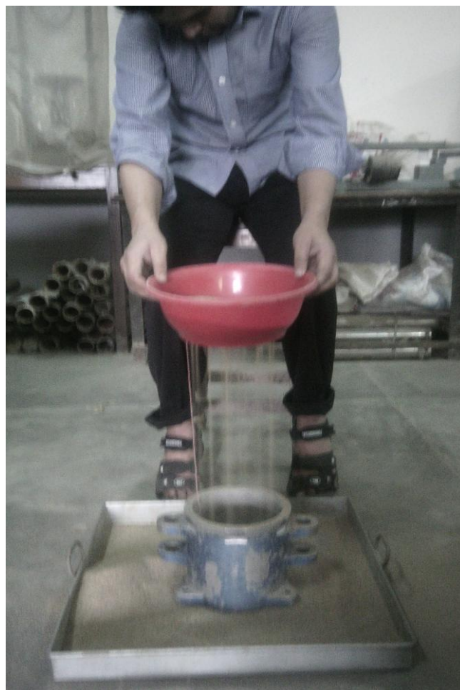
Fig. 3.4: Air pluviation method
