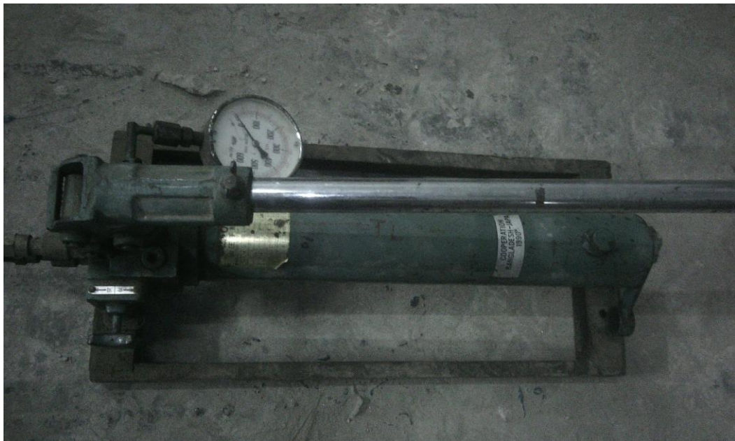
Fig. 3.14: Hydraulic pump and jack gauge
