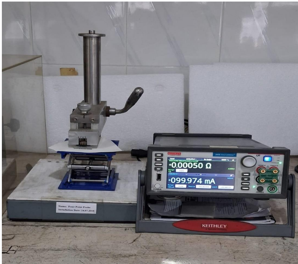
Figure 3.12: A photograph of the Homebuilt four-point collinear probe coupled with a Keithley SMU 2400 (IPD, BCSIR)
