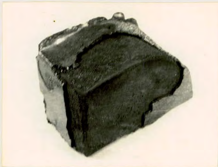
Fig.4.29: Oxidized at 1050-1100°C Fuel:air ratio =1:12 soaking time = 2 hrs.
