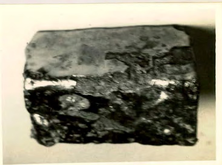
Fig.4.36: Oxidized at 1250- 1300°C Fuel : air ratio =1:12 soaking time = 3 hrs.
