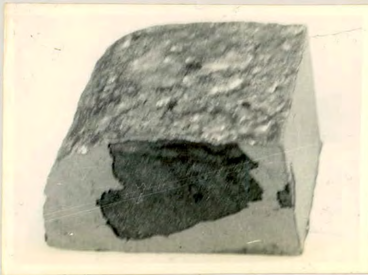
Fig.4.7: Oxidized at 1250-1300°C Fuel:air ratio =1:7 soaking time = 1 hr.
