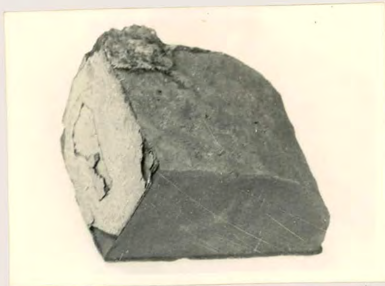
Fig.4.33: Oxidized at 1150-1200°C Fuel:air ratio =1:12 soaking time = 3 hrs.
