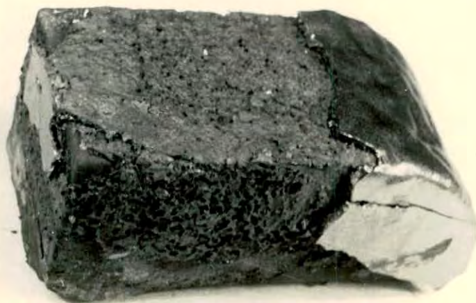
Fig.4.27: Oxidized at 1250-1300°C Fuel:air ratio =1:10 soaking time = 3 hrs.
