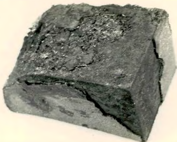
Fig.4.21: Oxidized at 1050-1100°C Fuel:air ratio =1:10 soaking time = 3 hr.
