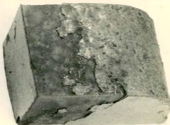
Fig.4.20: Oxidized at 1050- 1100°C Fuel : air ratio =1:10 soaking time = 2 hrs.
