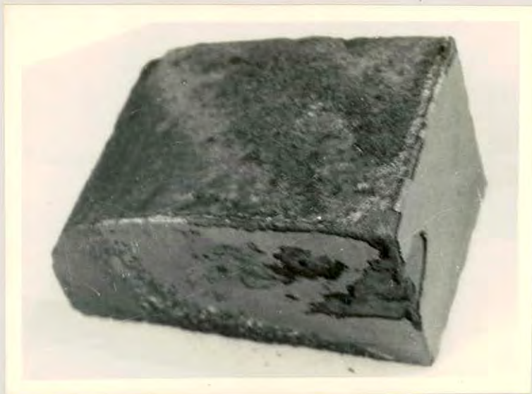
Fig.4.13: Oxidized at 1150-1200°C Fuel:air ratio =1:9 soaking time = 1 hr.
