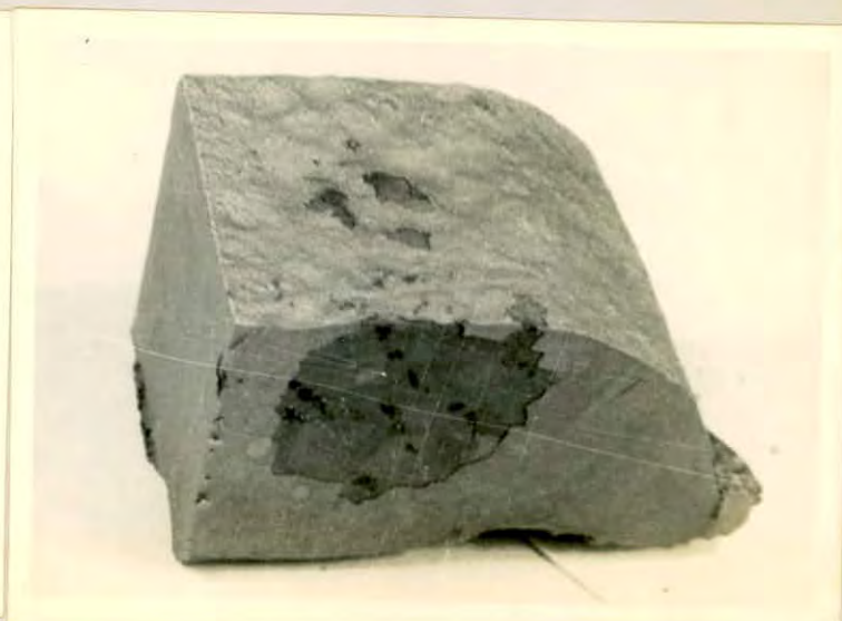
Fig.4.8: Oxidized at 1250- 1300°C Fuel : air ratio =1:7 soaking time = 2 hrs.
