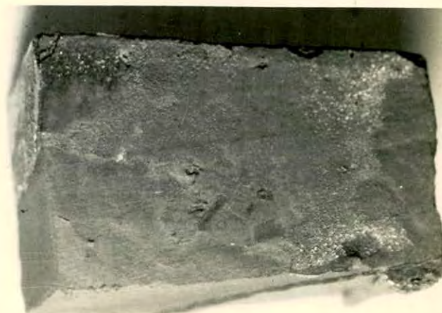
Fig.4.26: Oxidized at 1250- 1300°C Fuel : air ratio =1:10 soaking time = 2 hrs.
