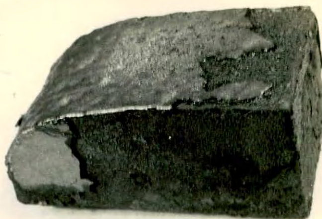
Fig.4.18: Oxidized at 1250- 1300°C Fuel : air ratio =1:9 soaking time = 3 hrs.
