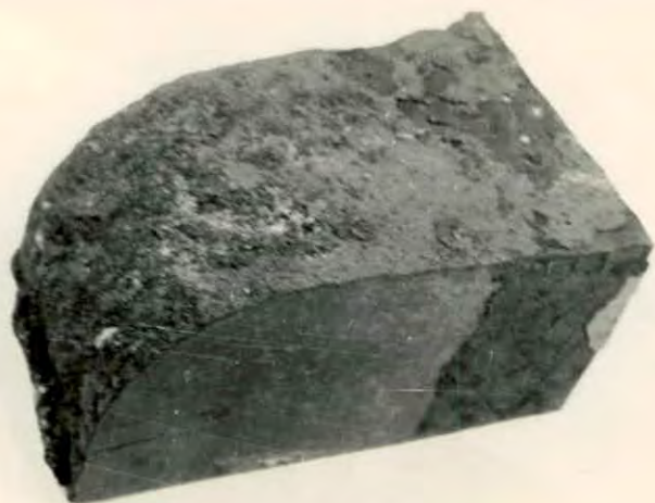
Fig.4.9: Oxidized at 1250-1300°C Fuel:air ratio =1:7 soaking time = 3 hrs.
