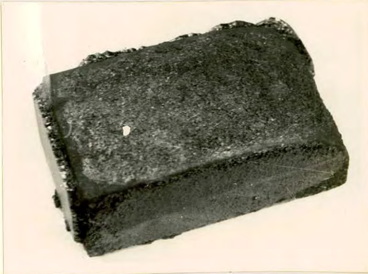
Fig.4.34: Oxidized at 1250- 1300°C Fuel : air ratio =1:12 soaking time = 1 hr.
