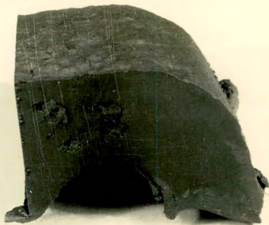
Fig.4.1: Oxidized at 1050-1100°C Fuel:air ratio =1:7 soaking time =1 hr.
