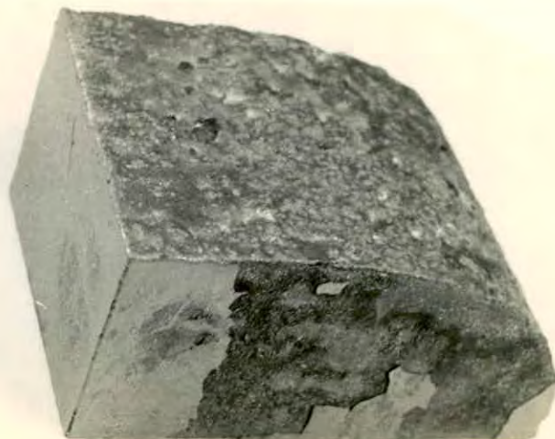
Fig.4.10: Oxidized at 1050- 1100°C Fuel : air ratio =1:9 soaking time = 1 hr.
