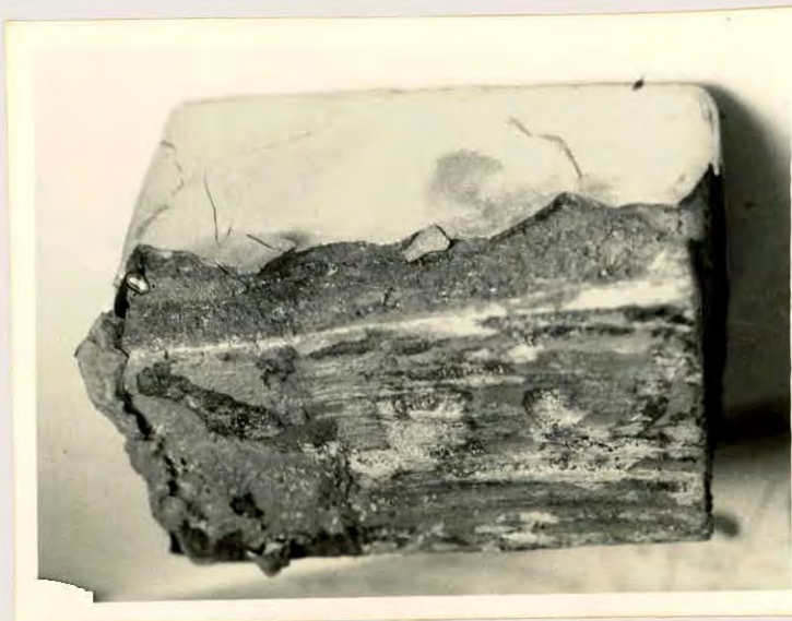
Fig.4.35: Oxidized at 1250-1300°C Fuel:air ratio =1:12 soaking time = 2 hrs.
