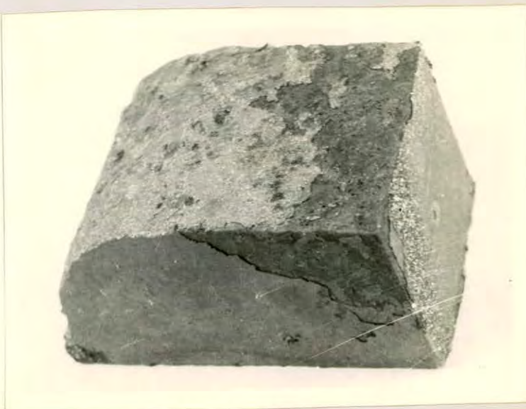
Fig.4.16: Oxidized at 1250- 1300 Fuel : air ratio= 1:9 soaking time = 1 hr.
