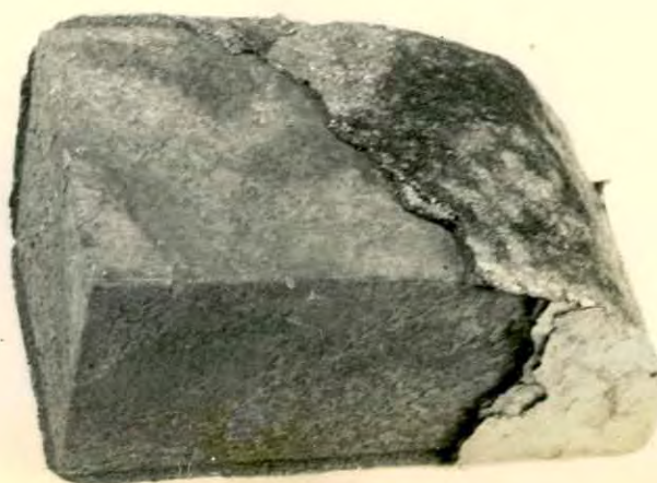
Fig.4.26: Oxidized at 1250- 1300°C Fuel : air ratio =1:10 soaking time = 2 hrs.
