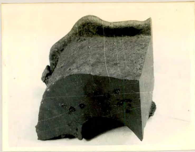
Fig.4.5: Oxidized at 1150-1200°C Fuel:air ratio =1:7 soaking time = 2 hrs.
