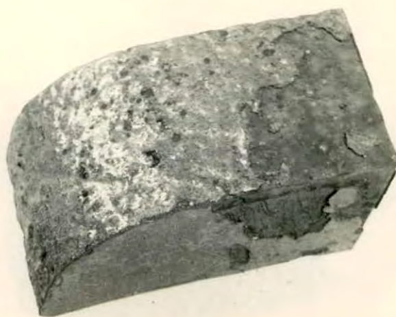
Fig.4.12: Oxidized at 1050- 1100°C Fuel : air ratio =1:9 soaking time = 3 hrs.
