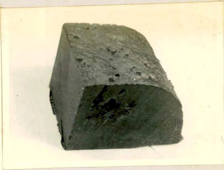
Fig.4.6: Oxidized at 1150- 1200°C Fuel : air ratio =1:7 soaking time = 3 hrs.
