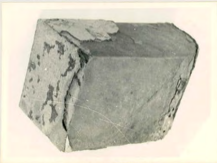
Fig.4.31: Oxidized at 1150-1200°C Fuel:air ratio =1:12 soaking time = 1 hr.
