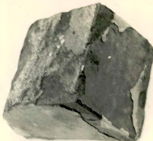
Fig.4.22: Oxidized at 1150- 1200°C Fuel : air ratio =1:10 soaking time = 1 hr.
