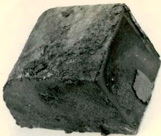
Fig.4.17: Oxidized at 1250-1300°C Fuel:air ratio =1:9 soaking time = 2 hrs.
