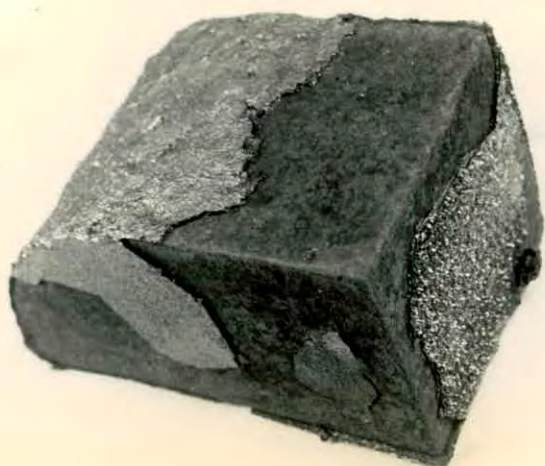
Fig.4.25: Oxidized at 1250-1300°C Fuel:air ratio =1:10 soaking time = 1 hr.
