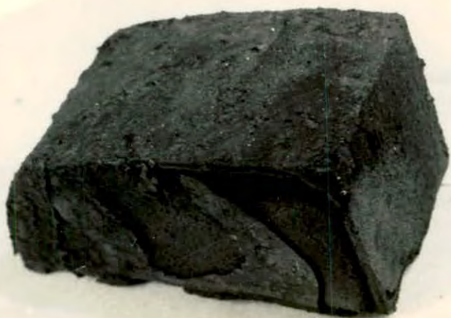
Fig.4.11: Oxidized at 1050-1100°C Fuel:air ratio =1:9 soaking time = 2 hrs.
