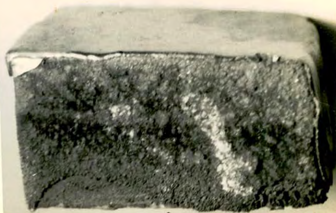
Fig.4.24: Oxidized at 1150- 1200°C Fuel : air ratio =1:10 soaking time = 3 hrs.
