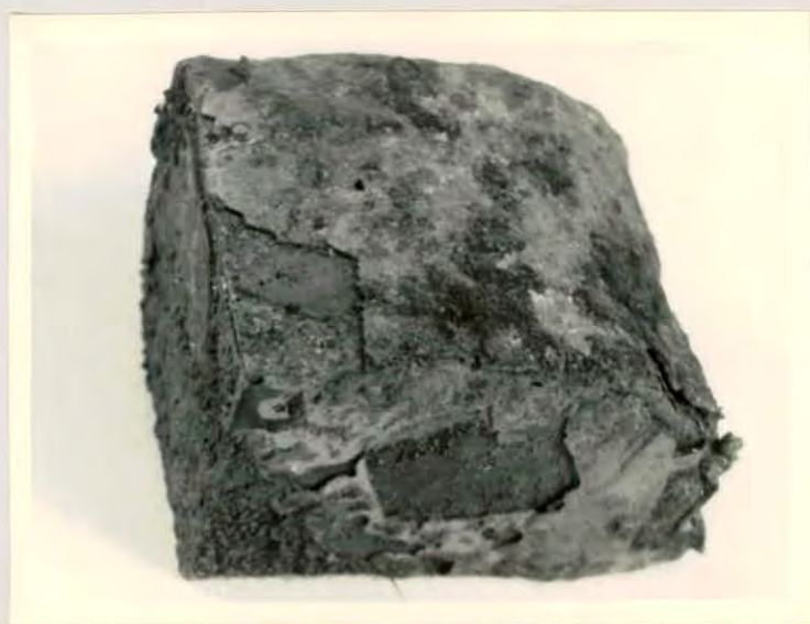
Fig.4.15: Oxidized at 1150-1200°C Fuel : air ratio =1:9 soaking time = 3 hrs
