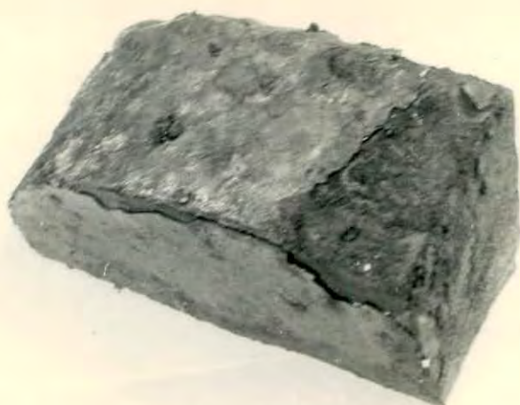
Fig.4.19: Oxidized at 1050-1100°C Fuel:air ratio =1:10 soaking time = 1 hr.
