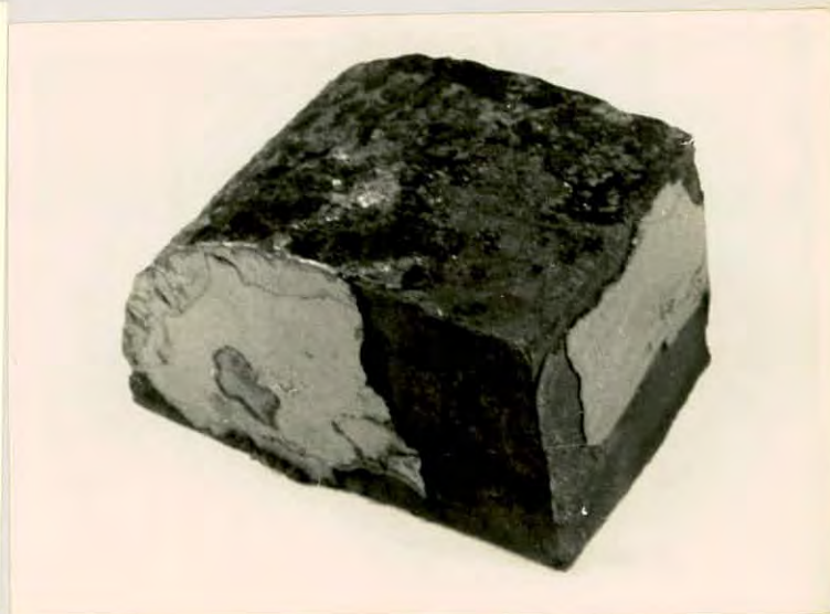
Fig.4.14: Oxidized at 1150- 1200°C Fuel : air ratio =1:9 soaking time = 2 hrs.
