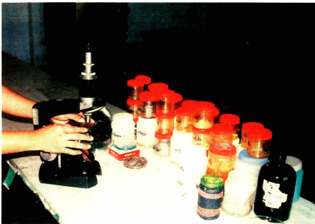
Photograph -12. Showing the examination of food contents under microscope with Sedgwick-Rafter cell
