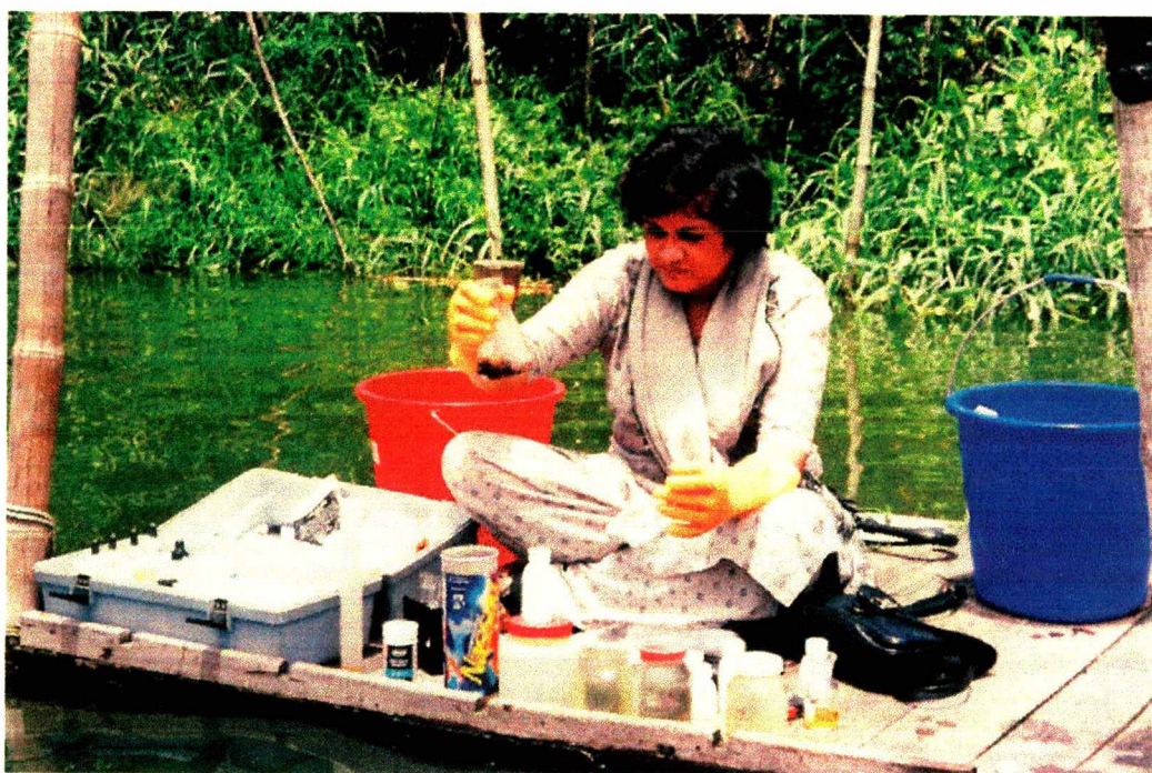
Photograph-4. Showing the researcher working with HACH KIT for determination of water quality parameters
