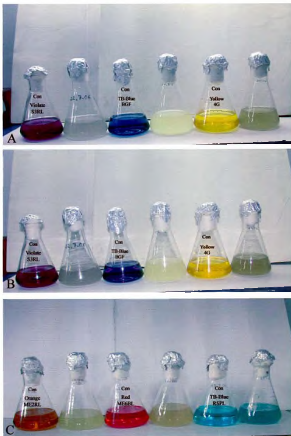
Fig. 3.7 (A-C) Photographs showing decolourization of selected dyes by using waste water sample. A, B. Violate S3RL, Turquoise Blue BGF and Yellow 4G and the waste water samples S-3 and S-9 respectively. C. Orange ME2RL, Red ME6BL and Turquoise Blue RSPL and the waste water sample S-4. (Con.- Control)
