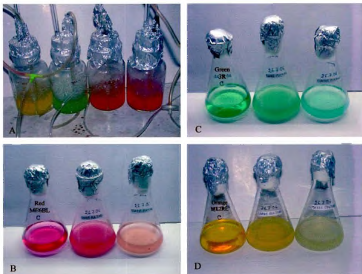
Fig. 3.8 (A-D) Photographs showing dye decolourization in three different conditions viz. static, shake and regular filtered aeration. C-Control.
