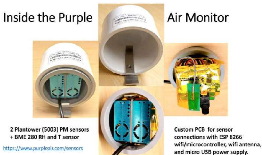
Figure D-1: Key elements of a PurpleAir \text{PM}_{2.5} sensor, specifically the sensor model: PAII SD. The figure is sourced from www.purpleair.com .
