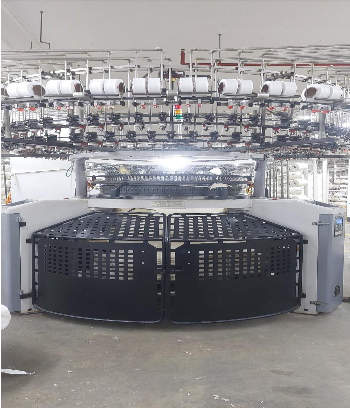
Fig2.4: Single jersey circular knitting machine
