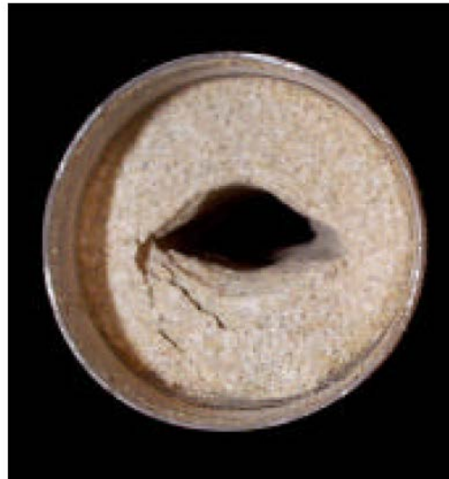
Hole collapse specimen after sample failure
