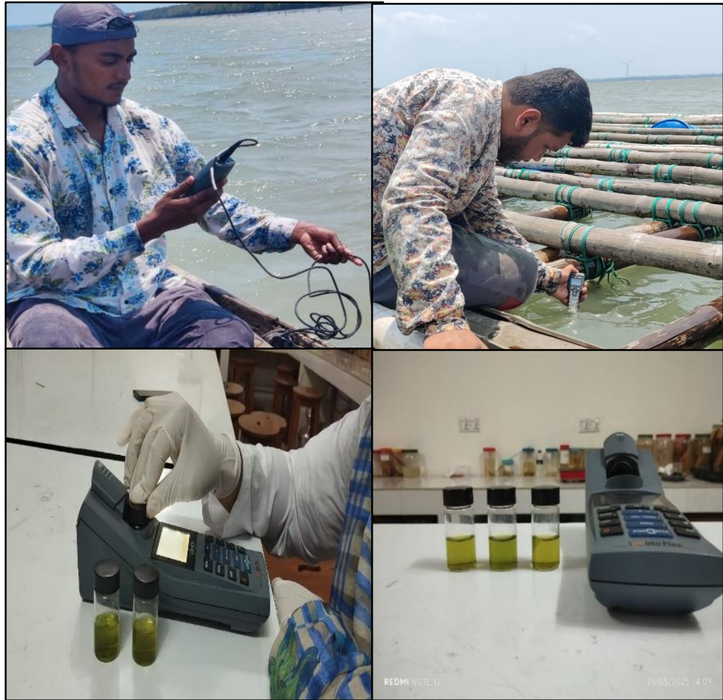
Figure 4: Measurement of water quality parameters from three depths & three locations monthly.
