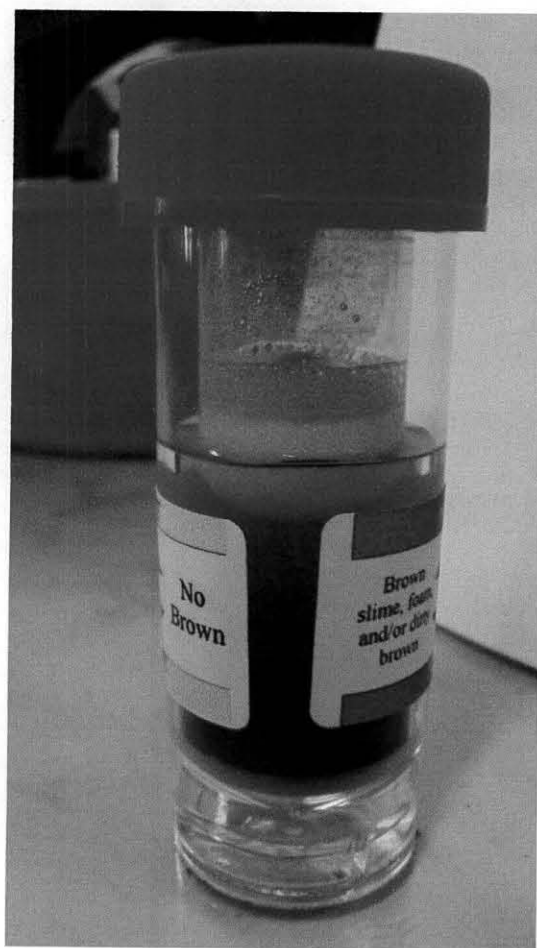
Figure 4.31 Presence of Anaerobic Bacteria (IRB) in raw groundwater of Batch C
