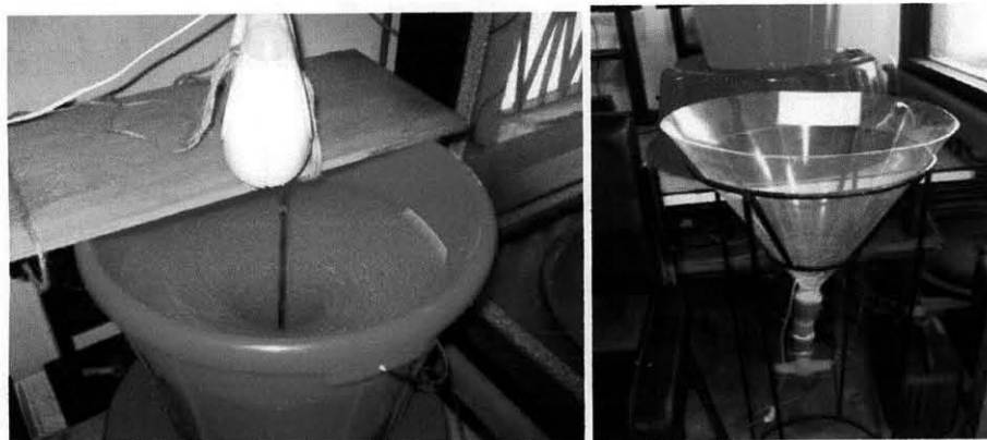
Figure 4.2 Mixing 20 liters of contaminated water with an electric kitchen mixer (left) and then run through the ten liter per hour prototype clarifier (right)
