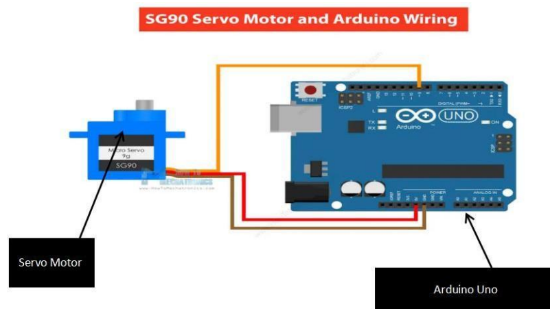
Figure 3.12: SG90 Servo Motor and Arduino Wiring
