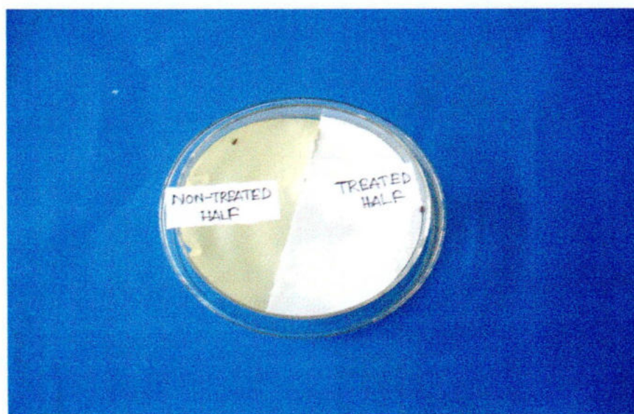
Plate 4 Repellency test of Bishkatali plant extract (with treated and untreated filter papers)
