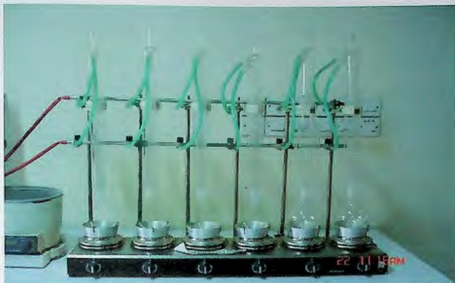
Plate 14 : Plant parts extraction in a Soxhlet's apparatus ( Type: EV-16 )
