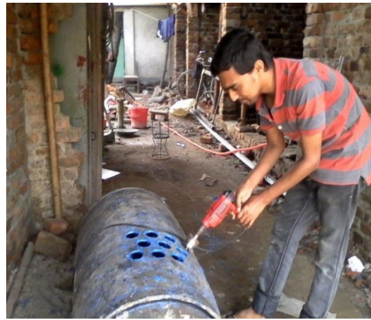
Fig-4: Making hole in the grading unit
