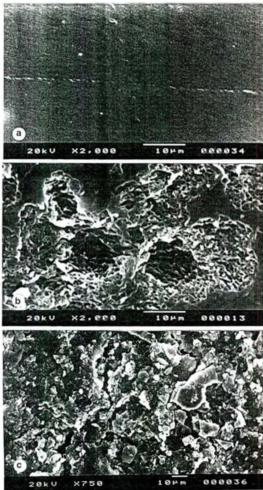
Fig. 3.9 (a-c): Scanning electron micrographs showing changes in surface morphology after prolonged soil exposure; (a) the control sample appeared as continuous sheet, (b) sample showing irregular cavities on film after 17 months and (c) fissures progressed with fragmentation after 22 months.
