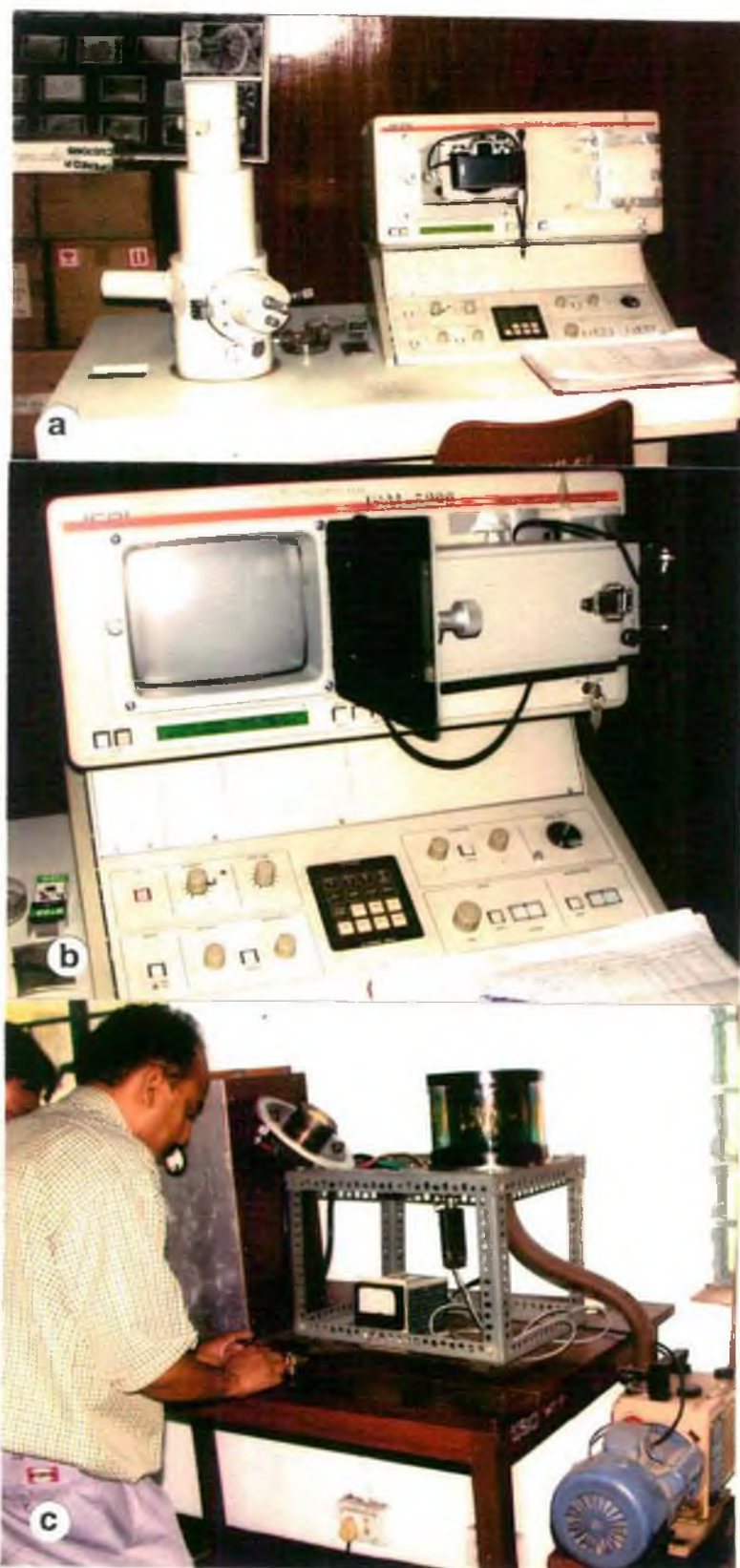
Fig. 3.5 (a-c): Photographs showing the SEM and shadow-casting equipments at the department of Instrumentation Science, Jadavpur University, India. (a) the Scanning Electron Microscope, (b) same showing the monitor screen, (c) the shadow casting equipment.
