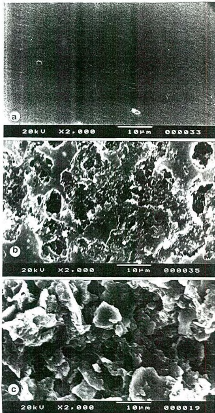
Fig. 3.6 (a-c): Scanning electron micrographs showing the structure and appearance of the sample no. 01 (PE w ) as revealed at 20 kV and x 2,000 (a) the control sample showing uniform and homogenous structure (b) numerous deeper holes formed after 17 months and (c) sample showing complete destruction of film integrity after 22 months. Loosening of portions is clearly visible.
