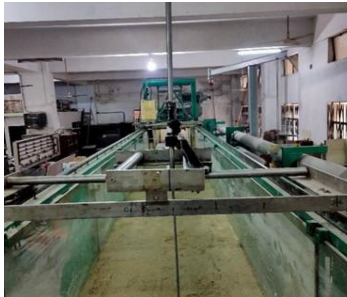
Figure 3.2 Vernier point gauge that measures the scour depth
