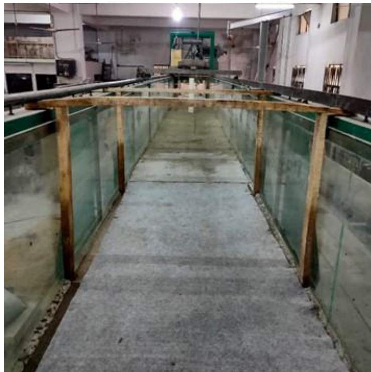
Figure 3.3 Modification of the flume with geotextile material on top.
