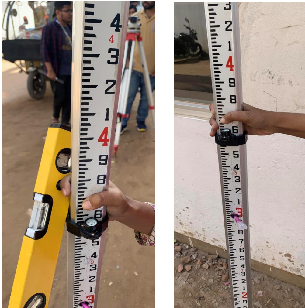
Figure 11 Scale which we are set up with bubble for perfect values.
