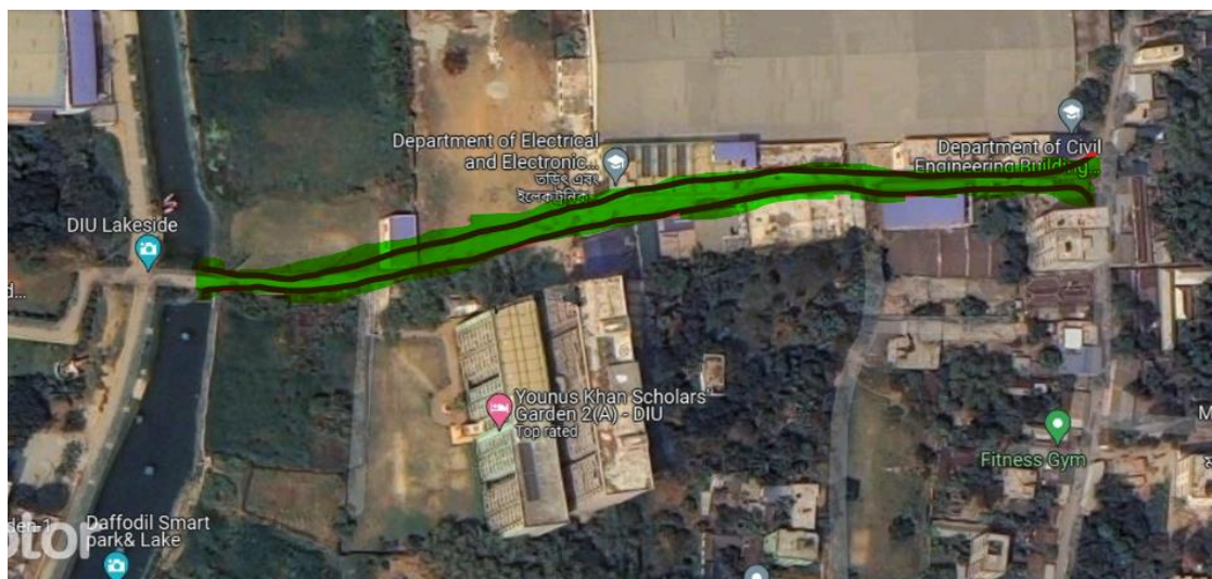
Figure 34 Pass through the rainfall water in the campus lake by constructing a drain.
