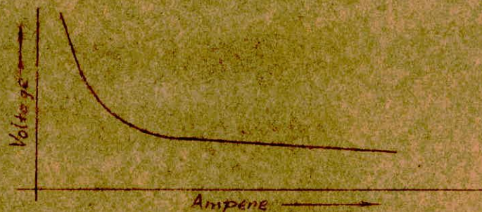
Fig. 8. Typical Volt-Ampere characteristic of arc.
