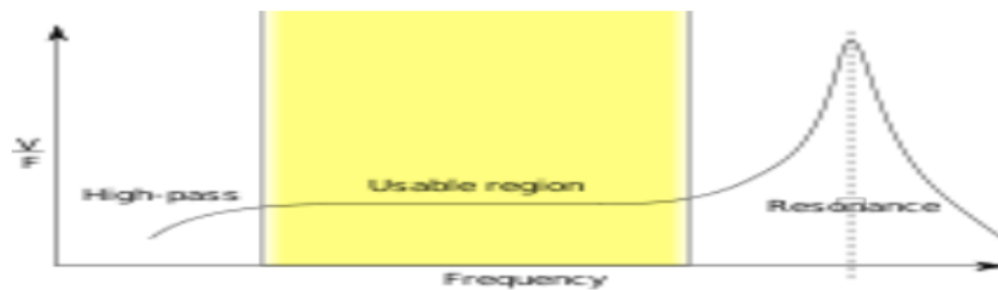
Fig 3.5 Frequency response of a piezoelectric sensor [5]
