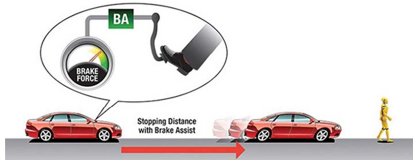
Figure 32. Braking Assist (BA) reduces stopping distance by up to 45% [35].
