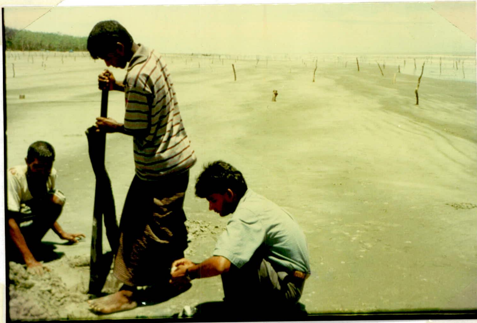
Photo 19: Collection of Soil Samples by hand scrapping at Station no. 1 (Chainage 0.00 Km)
