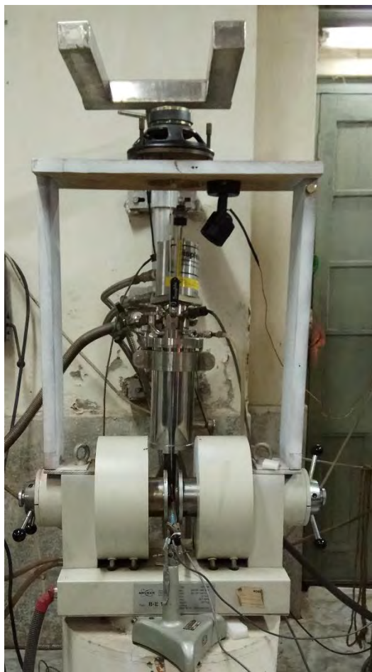
Figure 4.6 Vibrating Sample Magnetometer with PID Regulator (Materials Science Laboratory, Dept. of Physics, BUET)
