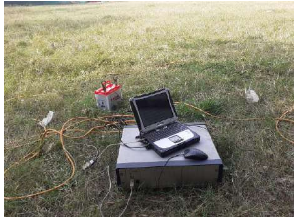
Microtremor at BH116
