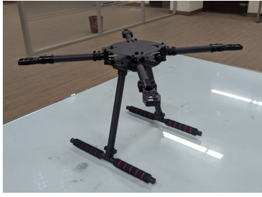
(a) Frame and Landing Gear
