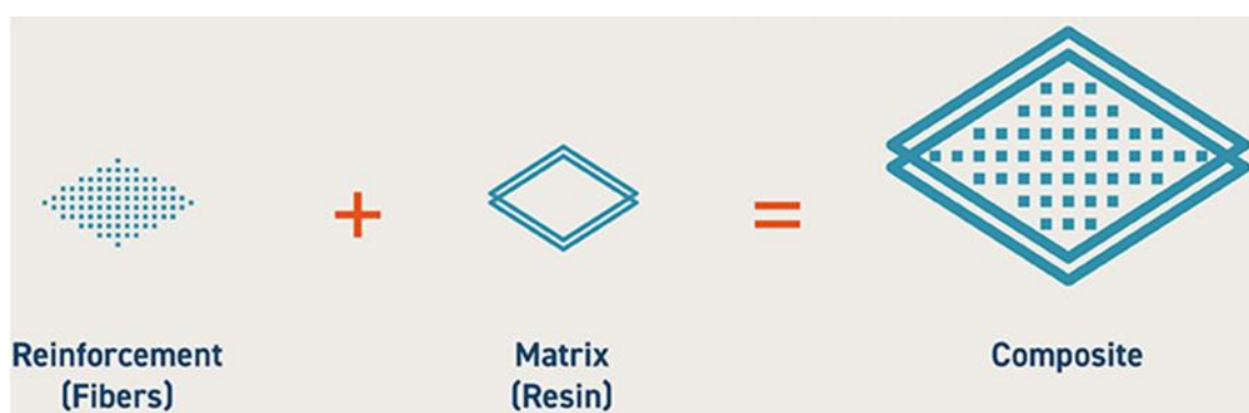
Figure 2.14 The above diagram depicts composites preparation.
