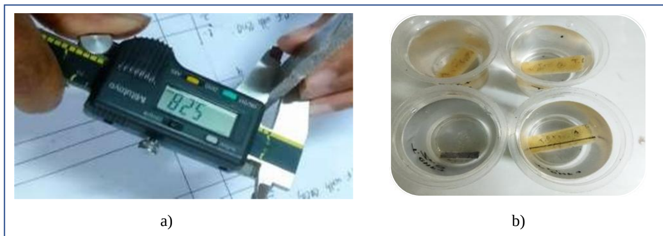
Figure 3.19: a) Measuring thickness by Digital slide scale b) Samples immersed in water
