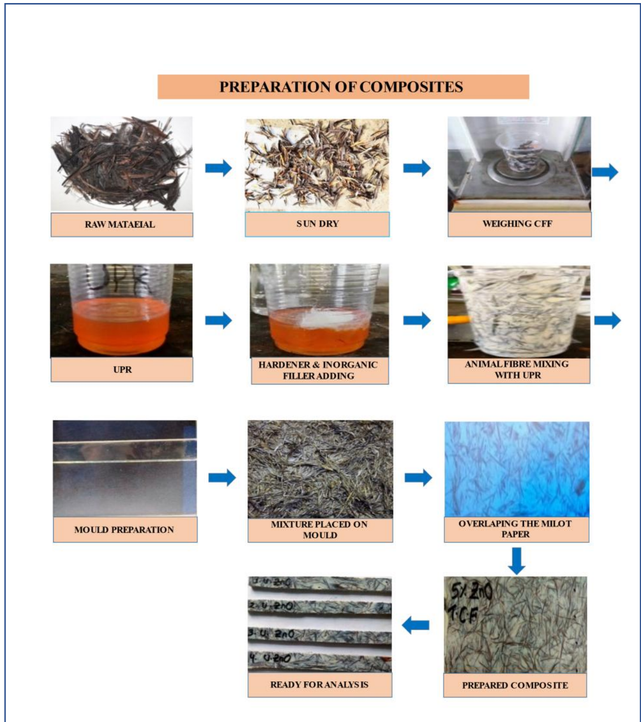
Figure 3.7: Preparation process of composite with image.
