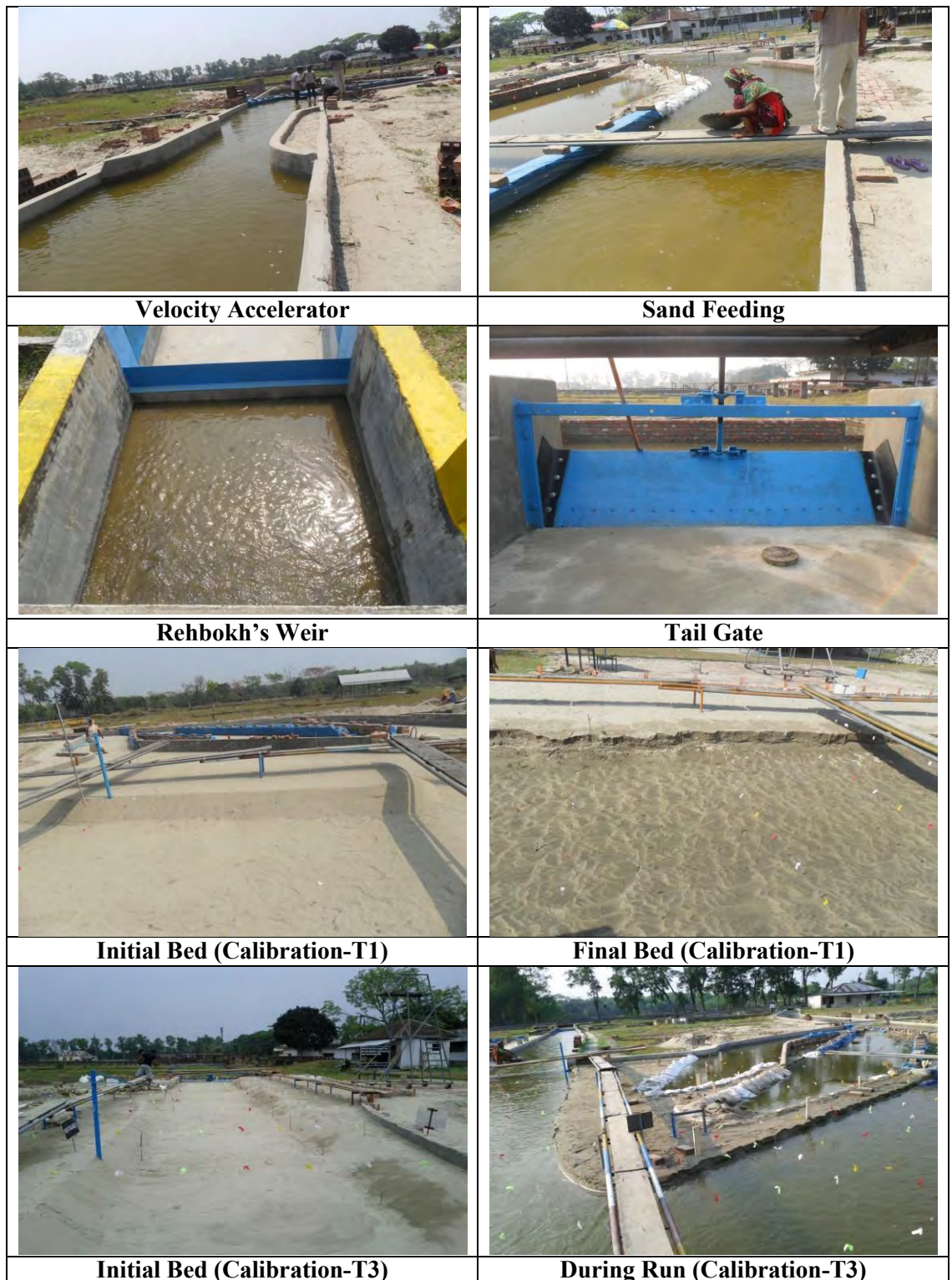
Figure A.3: Pictorial View of Model Run Setup at Different Conditions
