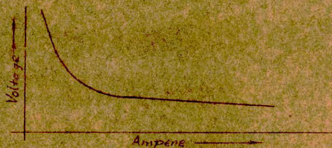
Fig. 8. Typical Volt-Ampere characteristic of arc.
