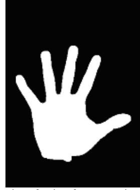
Fig. 4. Elimination of wrist after successive morphological operations
