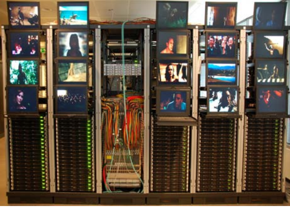
Figure 3. The iLab.t Virtual Wall consists of 100 identical server machines, 20 of them are connected to a monitor
