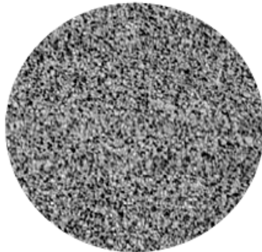
Fig. 8: Ferrite-pearlite microstructures of an ultra fine grain (UFG) structural steel.
