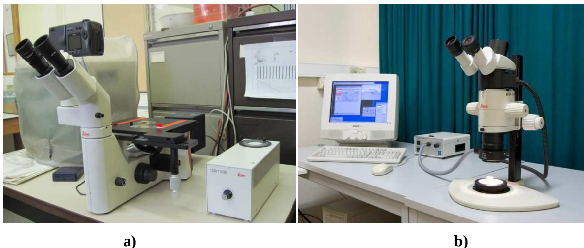
Figure 1: Optical microscopes, a) Leica CMD stereo microscope, b) Leica MZ8 image processing software based stereo optical microscope
