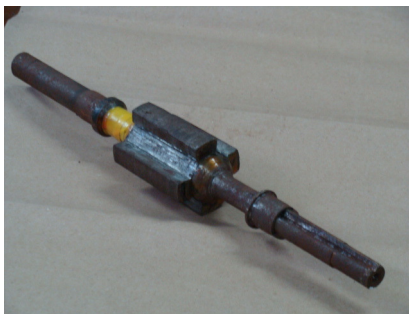
Fig. 2 Rotor turned in Lathe machine to remove squirrel cage winding
