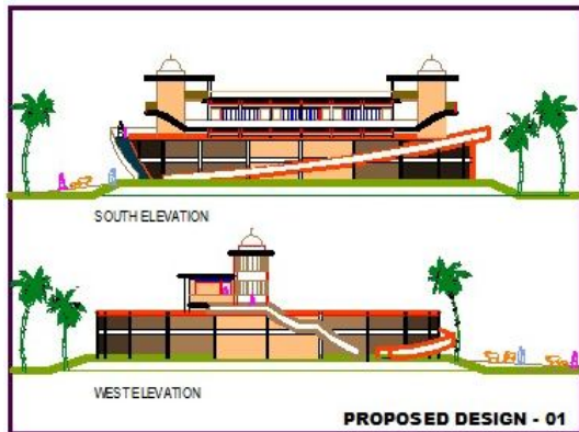
Fig. 14: Elevations showing the vertical circulation
