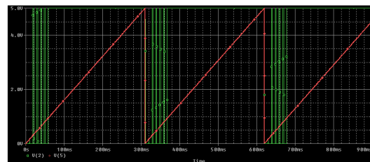
Fig 3: 1 st step simulation result from the MAGIC extraction file of the designed layout using PSpice.
