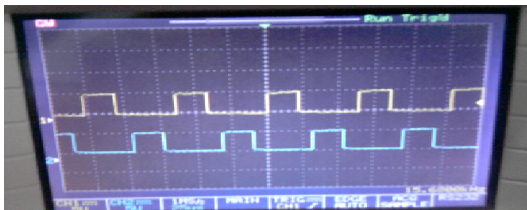
Fig. 7: MOSFET gate pulse with 70% duty cycle for medium load.
