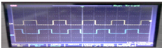
Fig. 9: MOSFET gate pulse with 90% duty cycle for maximum load.
