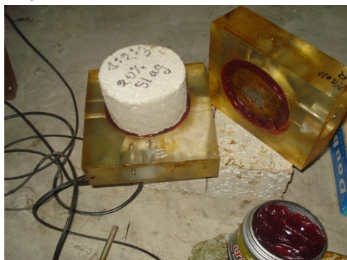
Fig. 1: Sealing of the sample with in the cell
