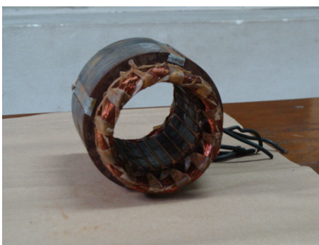
Fig. 7 Stator with coils inside the slots
