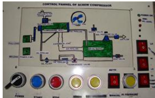
Fig. 5 Front view of the control panel of the screw air compressor
