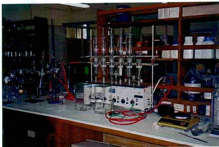
Fig. 33. Fat extracted through soxhlet apparatus
