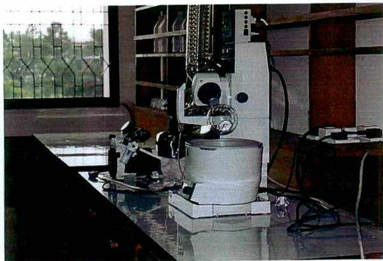
Fig. 35. Sample evaporated by Rotary Vacuum Evaporator
