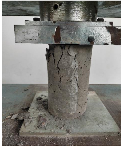
Fig. 3.11 Compressive Strength Test
