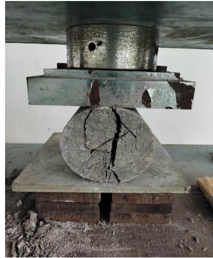
Fig. 3.12 Splitting Tensile Strength Test
