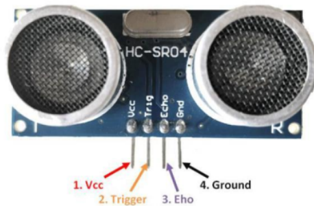
Fig 3.17: Pin Diagram of HC-SR04 Ultrasonic Sensor [47]
