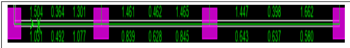
Figure 5.37 Steel Area of 3 rd Floor Beam X-axis
