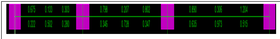
Figure 5.61 Steel Area of Roof Floor Beam X-axis
