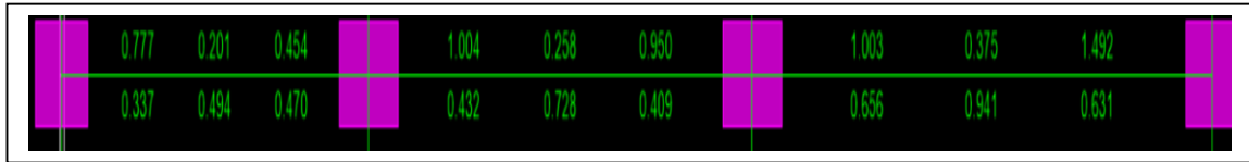
Figure 5.57 Steel Area of 8 th Floor Beam X-axis
