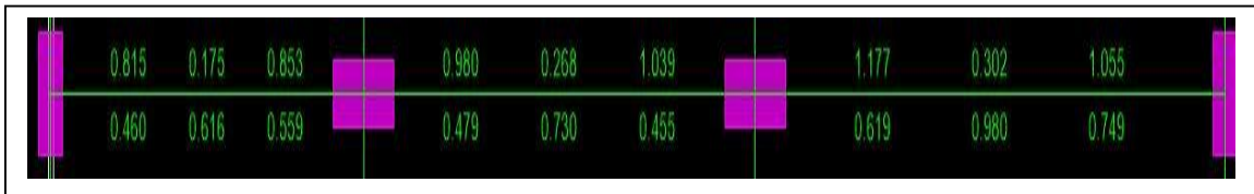
Figure 5.13 Steel Area of 3 rd Floor Beam X-axis
