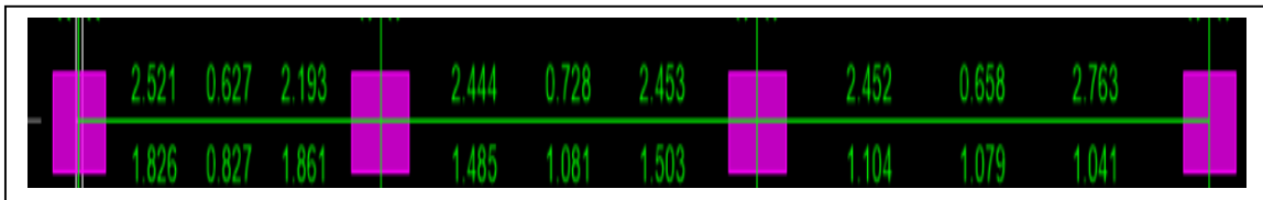
Figure 5.33 Steel Area of 2 nd Floor Beam X-axis
