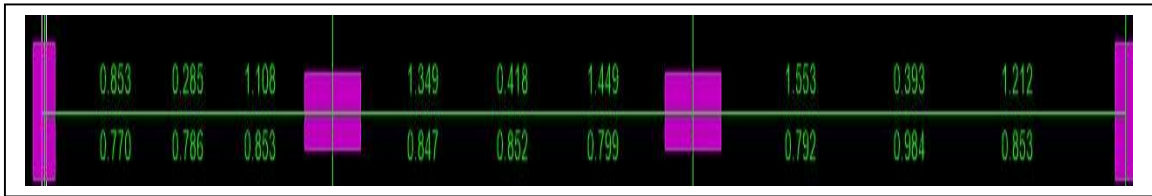
Figure 5.5 Steel Area of 1 st Floor Beam X-axis
