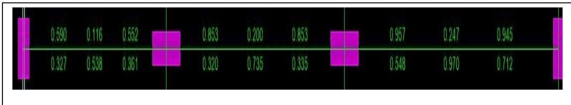
Figure 5.17 Steel Area of 4 th Floor Beam X-axis
