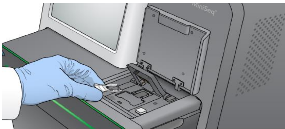
Figure 5: Place Flow Cell on Stage
