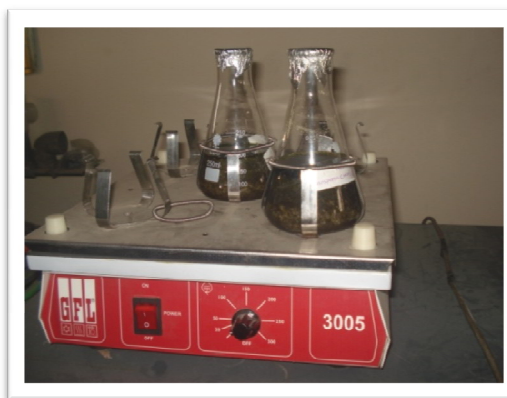
Plate 2.3: Plunged samples in conical flasks on a shaker
