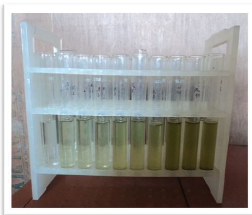
Plate 2.15: Bioassay with plant extracts on A. salina nauplii by brine shrimp lethality test
