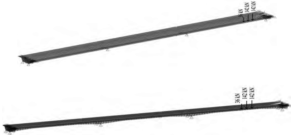
Figure 3.11A: Finite Element Model Including Vehicle Load at Cantilever Part
