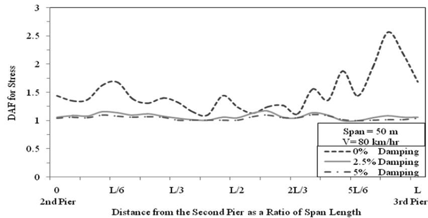
Fig B1.33 : DAF for Stress for 50 m Span Length and V = 80 km/hr
