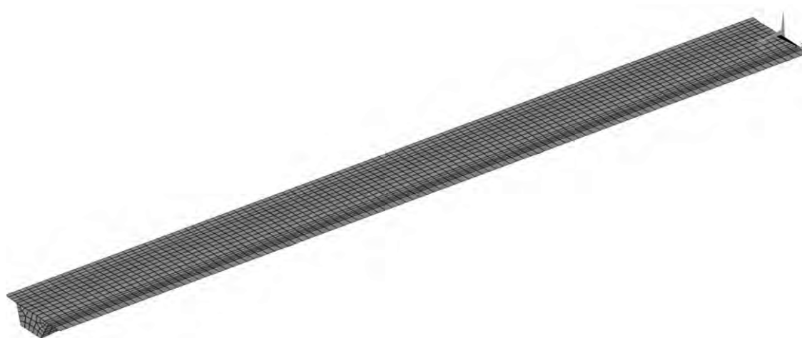
Figure 3.3: Finite Element Model of Box Girder Bridge
