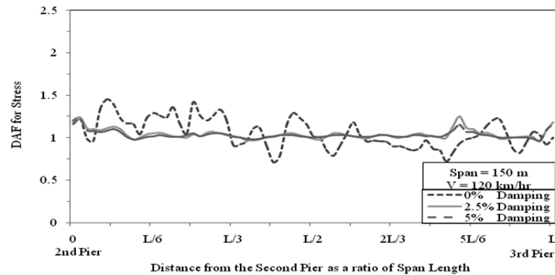
Fig B1.59 : DAF for Stress for 150 m Span Length and V = 120 km/hr
