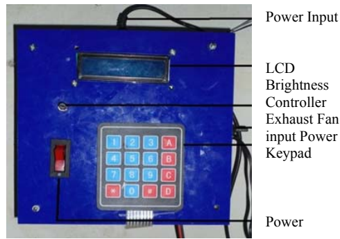
Fig. 5. Spray-dry control unit box
