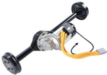
Figure 18. BLDC motor connected with rear wheel [9]
