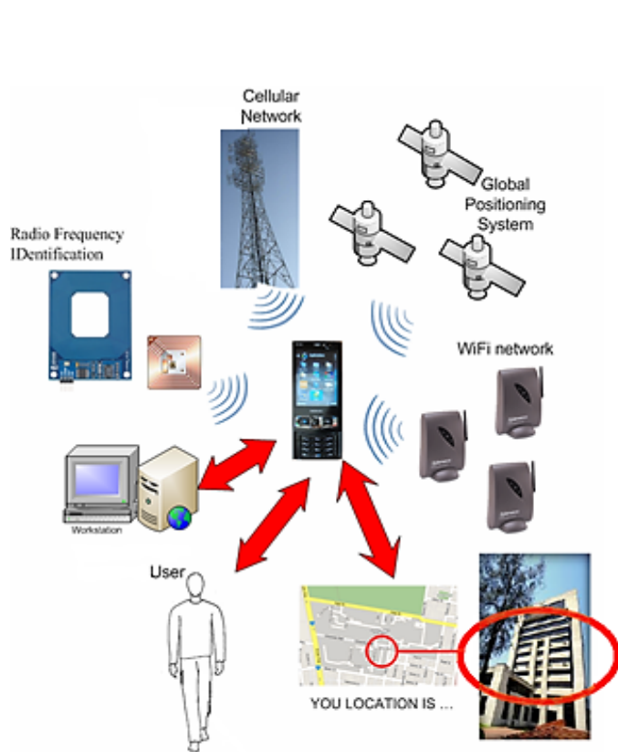
Fig. 3. Integrate several positioning technologies to provide location.
