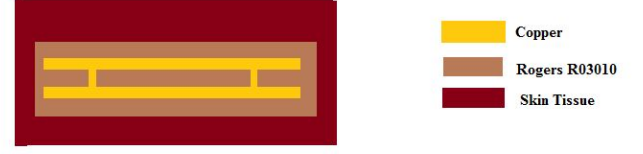
Fig. 2. Cross-sectional view of one layer skin model geometry of the antenna In Fig. 2, the antenna in the vicinity of human skin tissue is presented for a better understanding of the placement of antenna. Table I summarizes the antenna size parameters.
