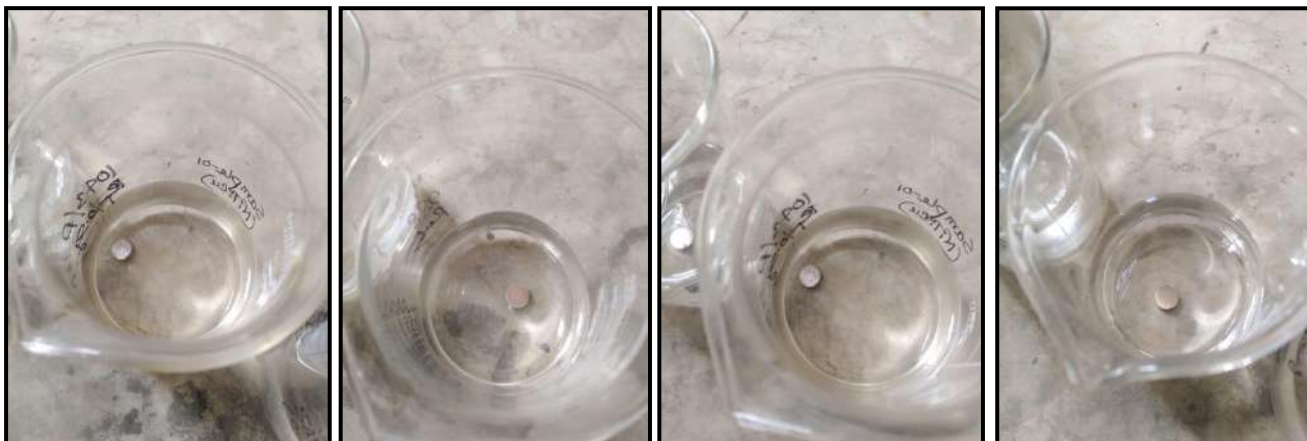
Figure 4.4: CuAlNi and NiTiCu submerged in PBS solution before corrosion
