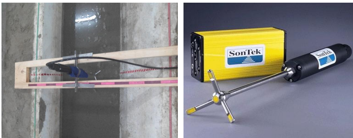
Figure 4.15 (a): Acoustic Doppler Velocimeter (ADV)
