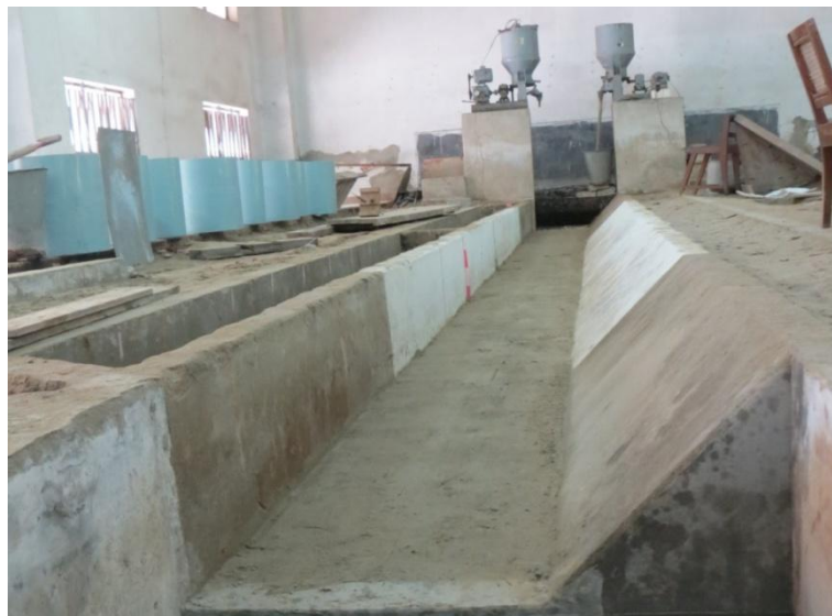
Figure 4.1: Sand bed channel at Hydraulics and River Engineering Laboratory, DWRE, BUET
