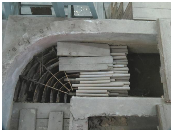
Figure 4.10: Guiding vanes and tubes
