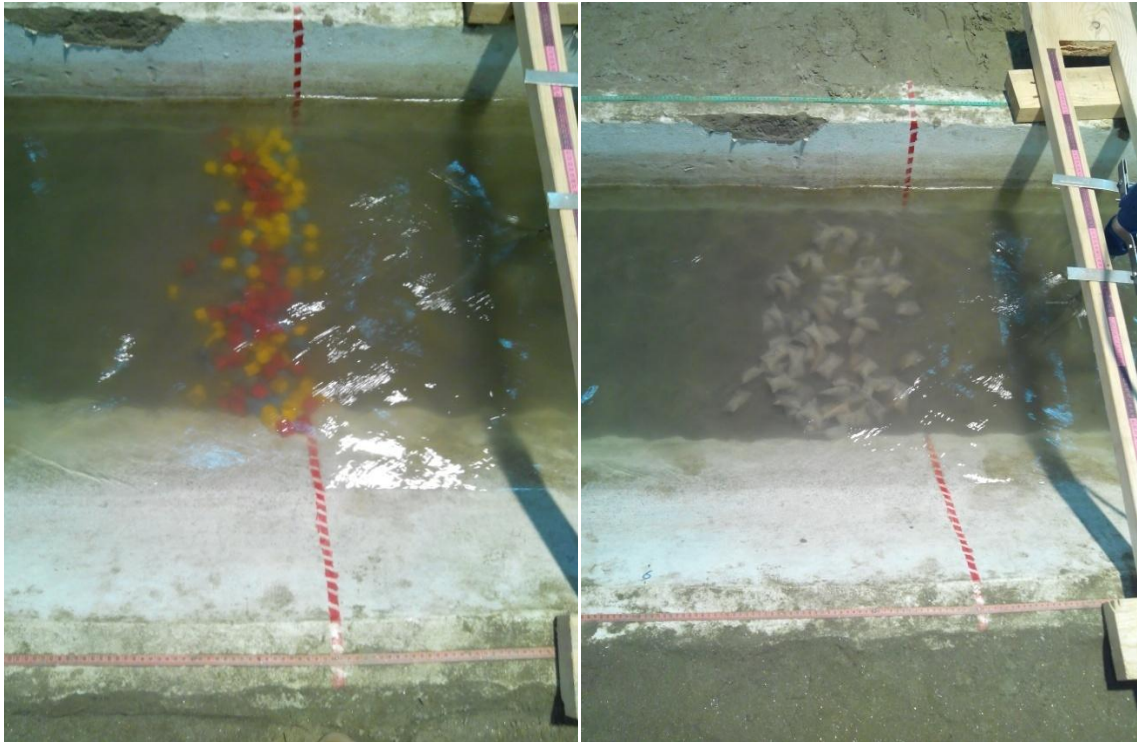
Figure 4.19: Investigation of placement of falling apron (CC blocks and Geobags)
