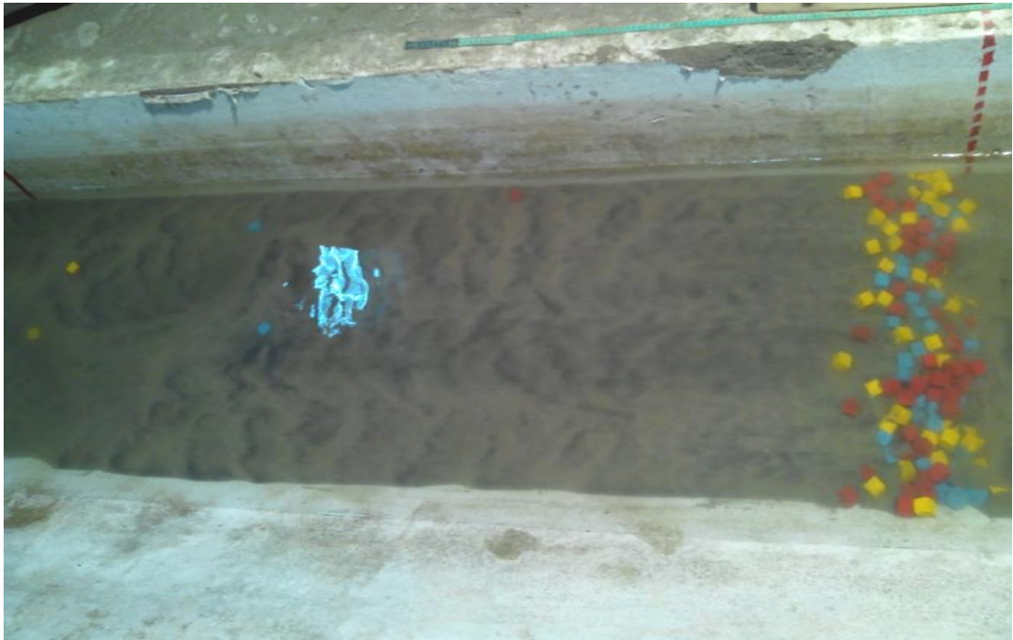
Figure 4.20: Displacement of CC blocks at incipient condition (Underwater construction)
