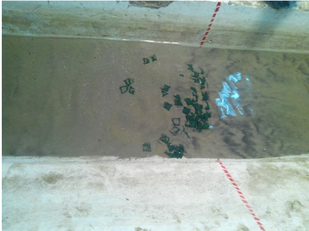
Figure 4.23: Displacement of geobags at incipient condition (Dry bed condition)
