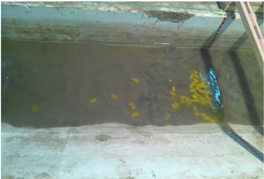
Figure 4.21: Displacement of geobags at incipient condition (Underwater construction)
