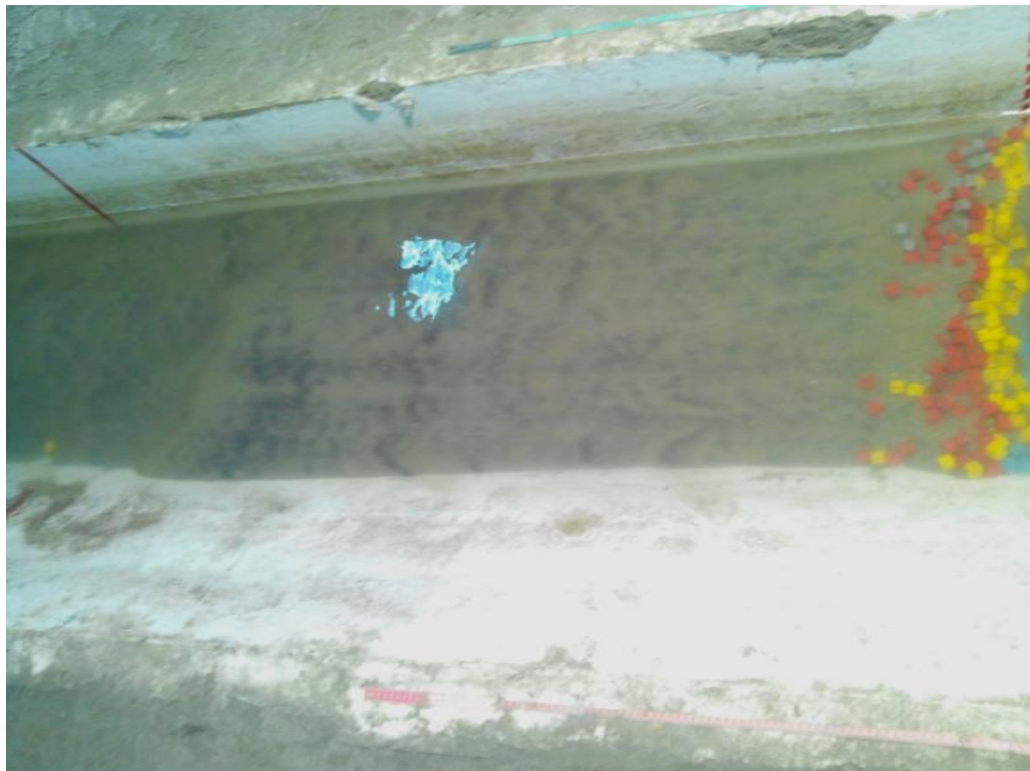
Figure 4.22: Displacement of CC blocks at incipient condition (Dry bed Condition)
