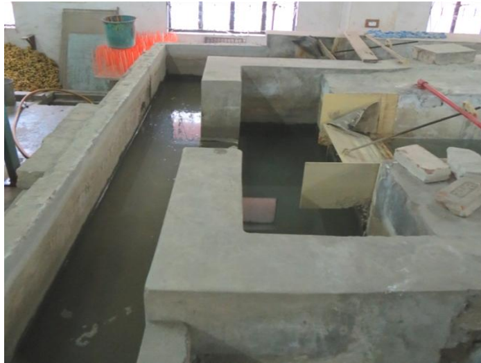
Figure 4.9: Stilling basin and transition flumes
