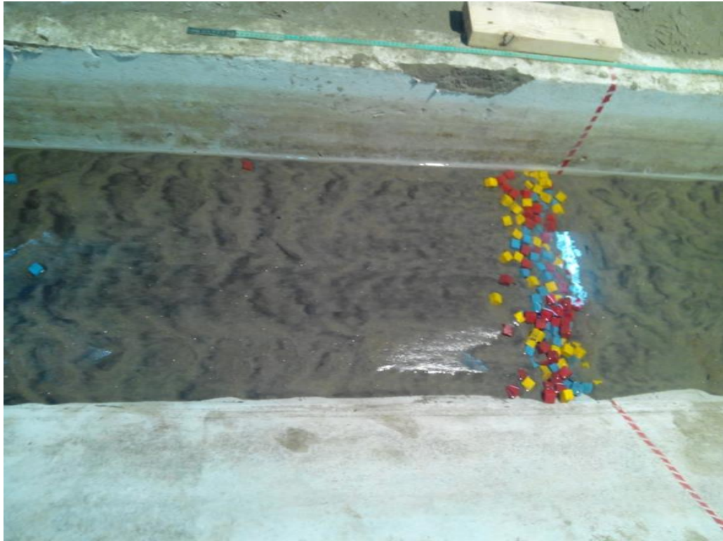
Figure 4.24: Bed form during the experimentation
