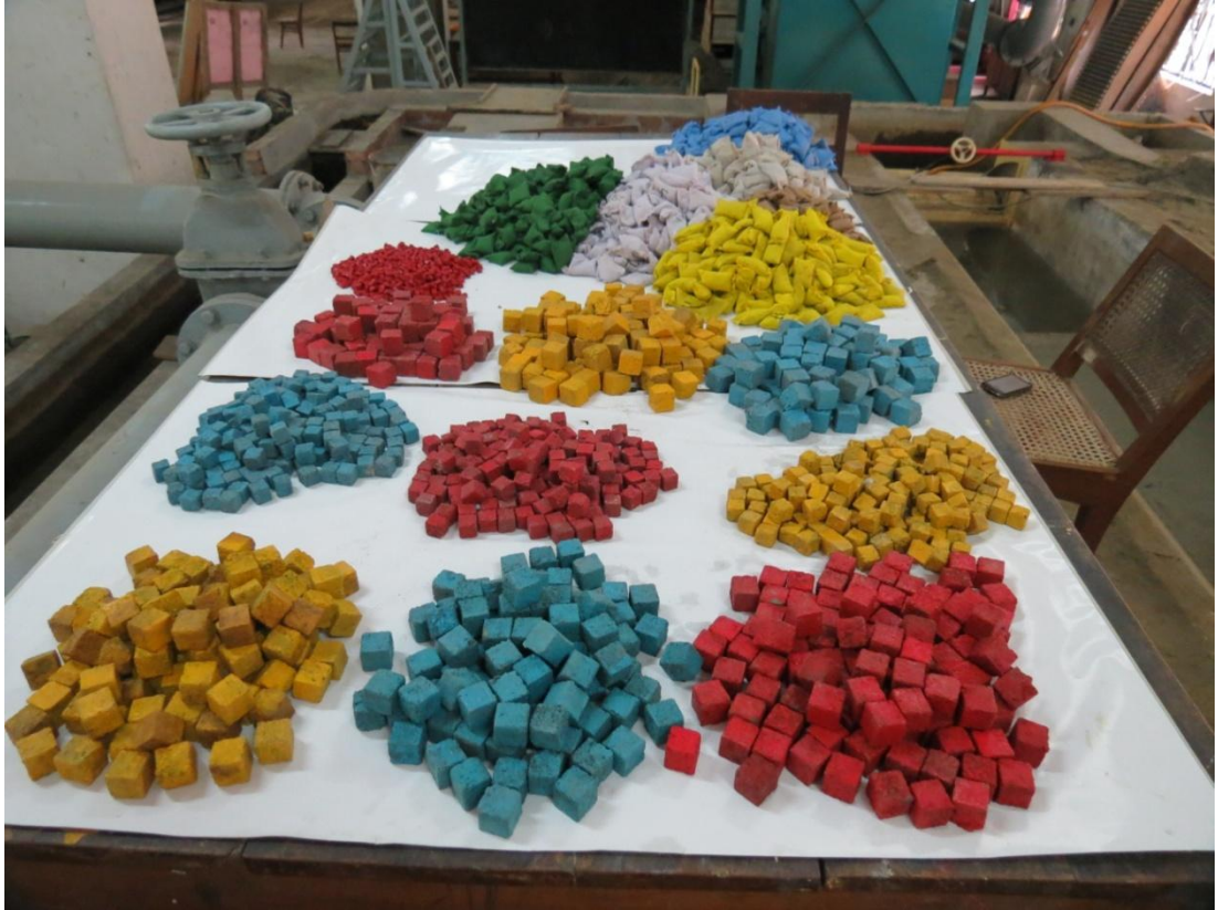
Figure 4.16: CC blocks and geobags used in the experiment
