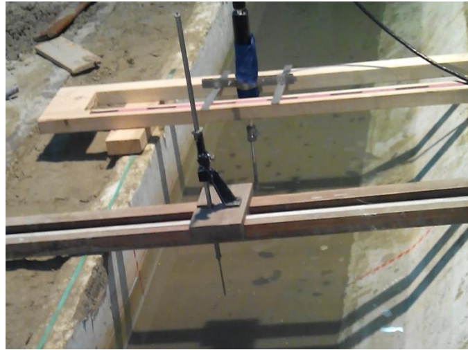
Figure 4.14: Point gage and measuring bridge
