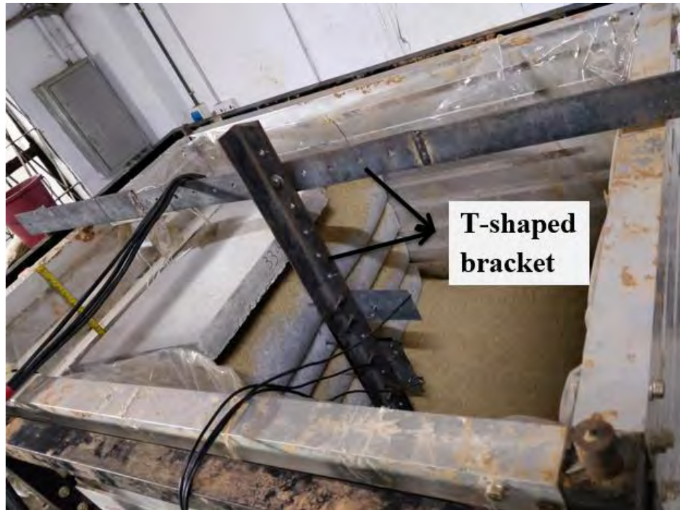
Figure 4.15: T-shaped bracket for supporting LVDTs.
