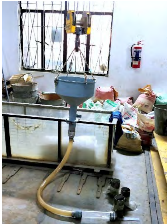
Figure 4.2 c: Portable pluviator for construction of the model wall.
