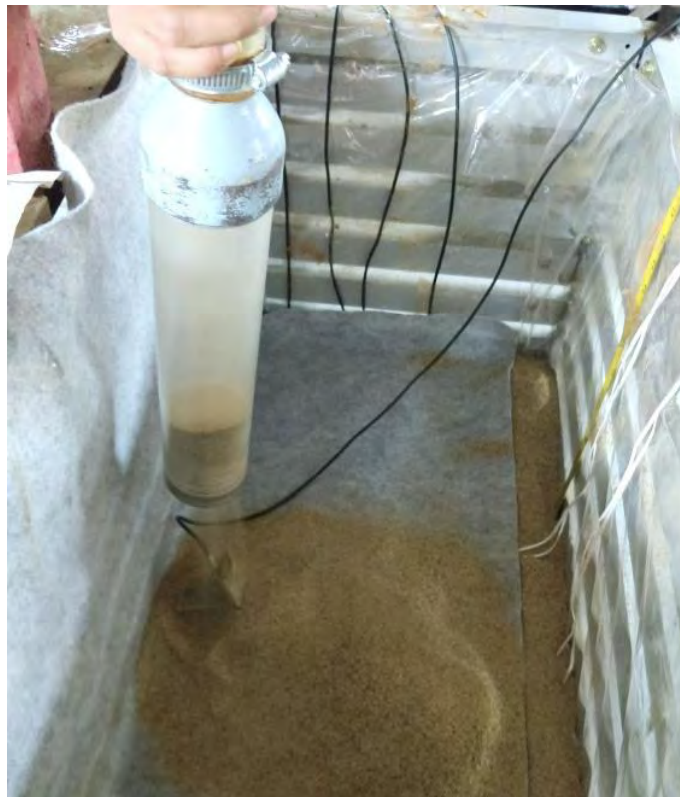
Figure 4.17: Attached scale with diffuser to maintain accurate height of fall.
