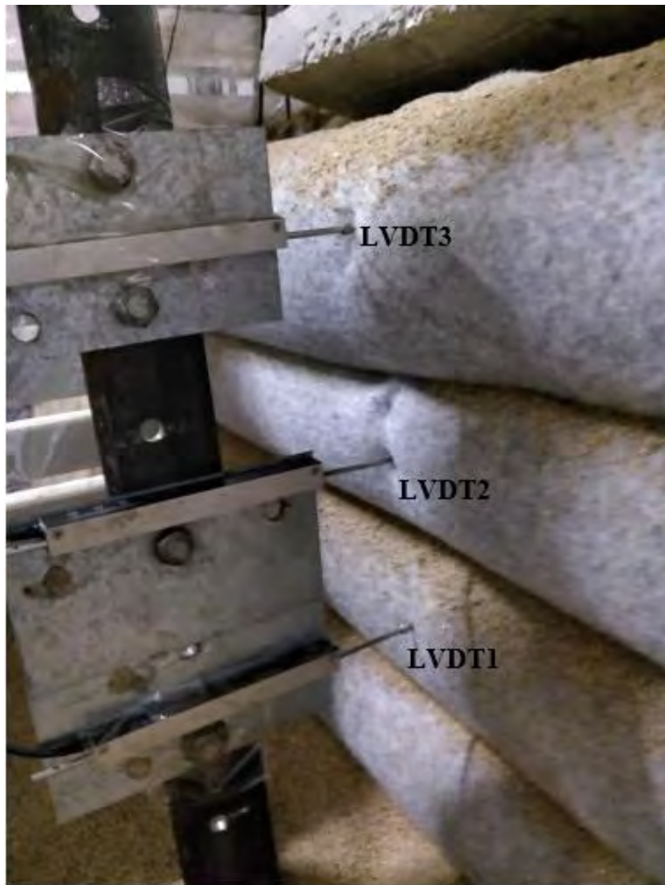
Figure 4.14: Three allocated LVDTs.
