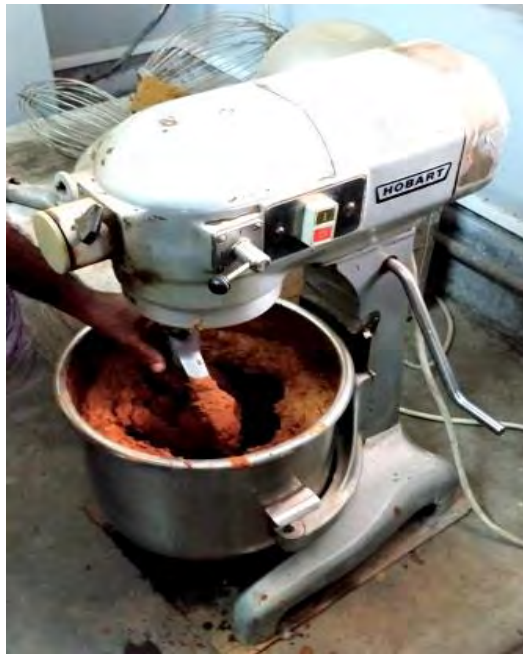
Figure 4.4. a) The mixing process of slurry with Hobart rotary mixer
