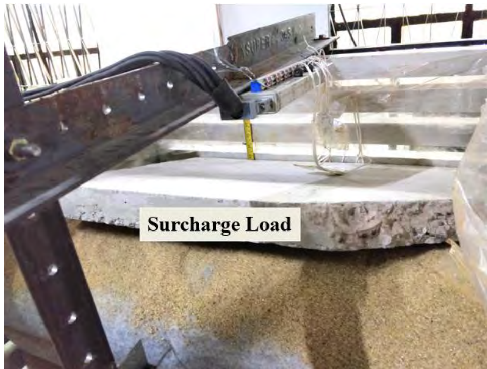
Figure 4.15: T-shaped bracket for supporting LVDTs.
