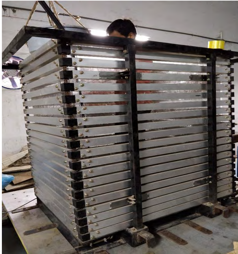
Figure 4.2a: Laminar box mounted on the shaking platform.
