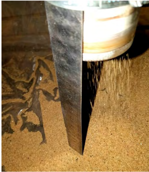
Figure 4.17: Attached scale with diffuser to maintain accurate height of fall.
