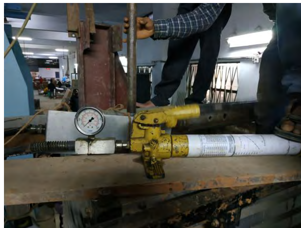
Figure 4.9 (b): conducting CPT test on Reconstitute soil sample
