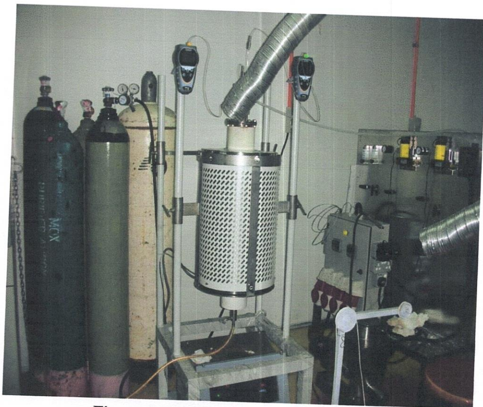
Figure 4.23. Ten liter volume activation reactor.
