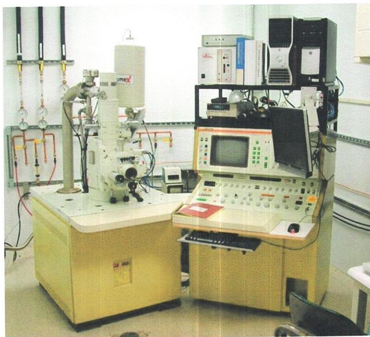
Figure 4.12. Scanning Electron Microscope (SEM) used for morphological study of activated carbons.
