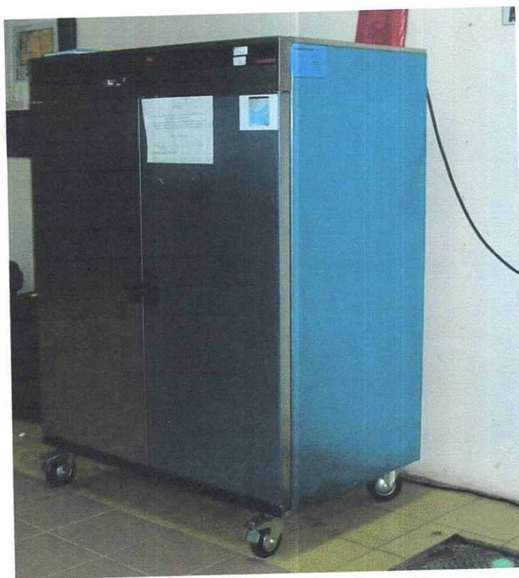
Figure 4.5. Oven (Model – OV445) used for drying feedstock and product sample
