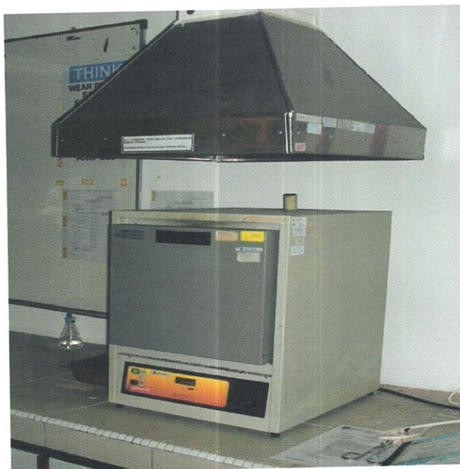
Figure 4.6. Muffle furnace for calcination and ash content determination.
