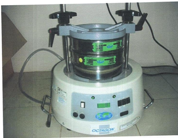
Figure 4.3. Standard testing sieve loaded on a shaker for jute stick screening.
