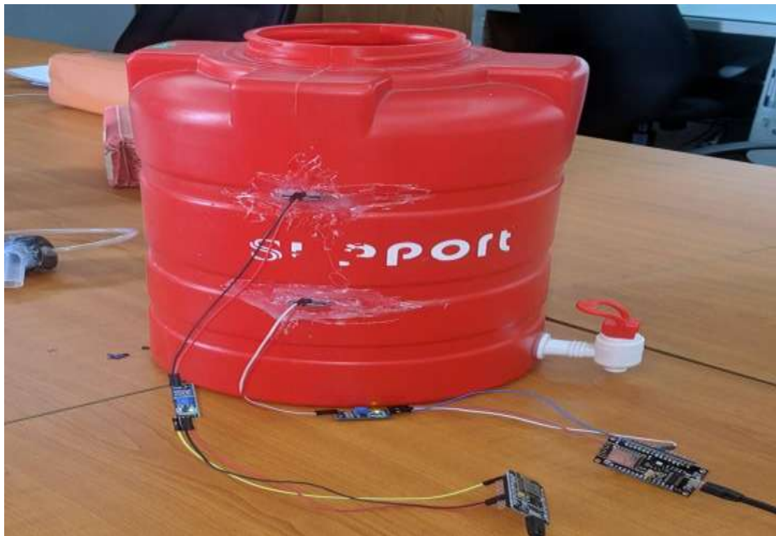
Figure 5.4: Sensor and NodeMCU module for receiving data
