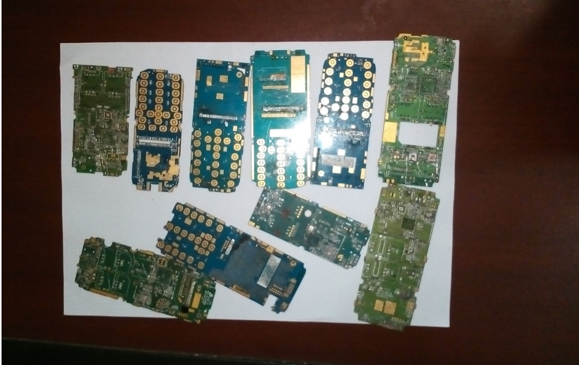
Figure 3.2: Surfaces of MPCBs after removing the tiny parts
