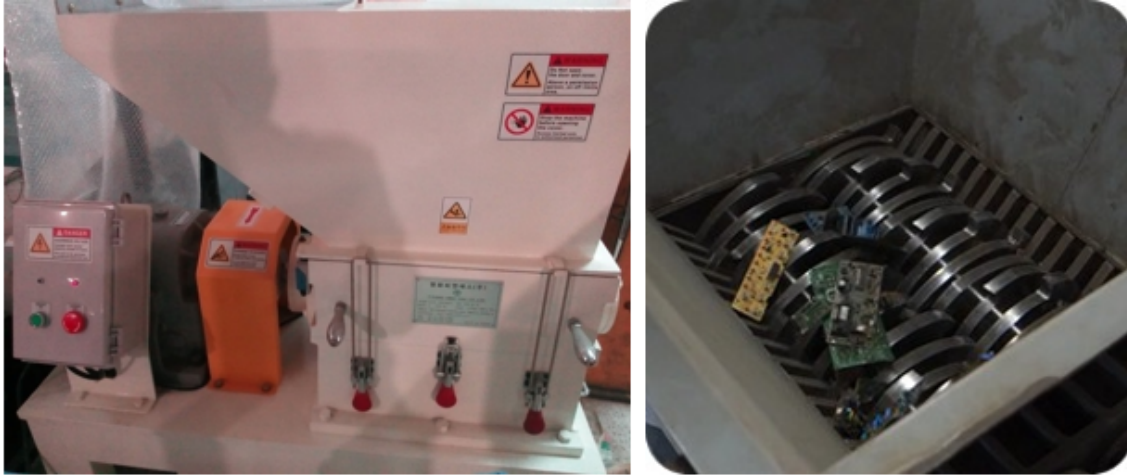
Figure 3.3: Shredder used for size reduction
