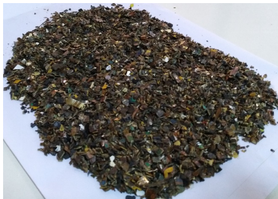
(b) \text{HNO}_3 treated air dried PCB sample
