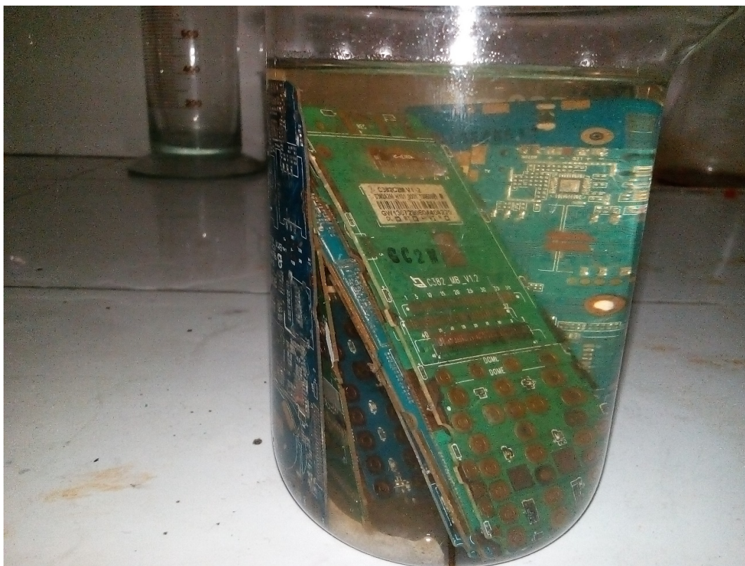
Figure 3.5: NaOH treatment of whole PCB
