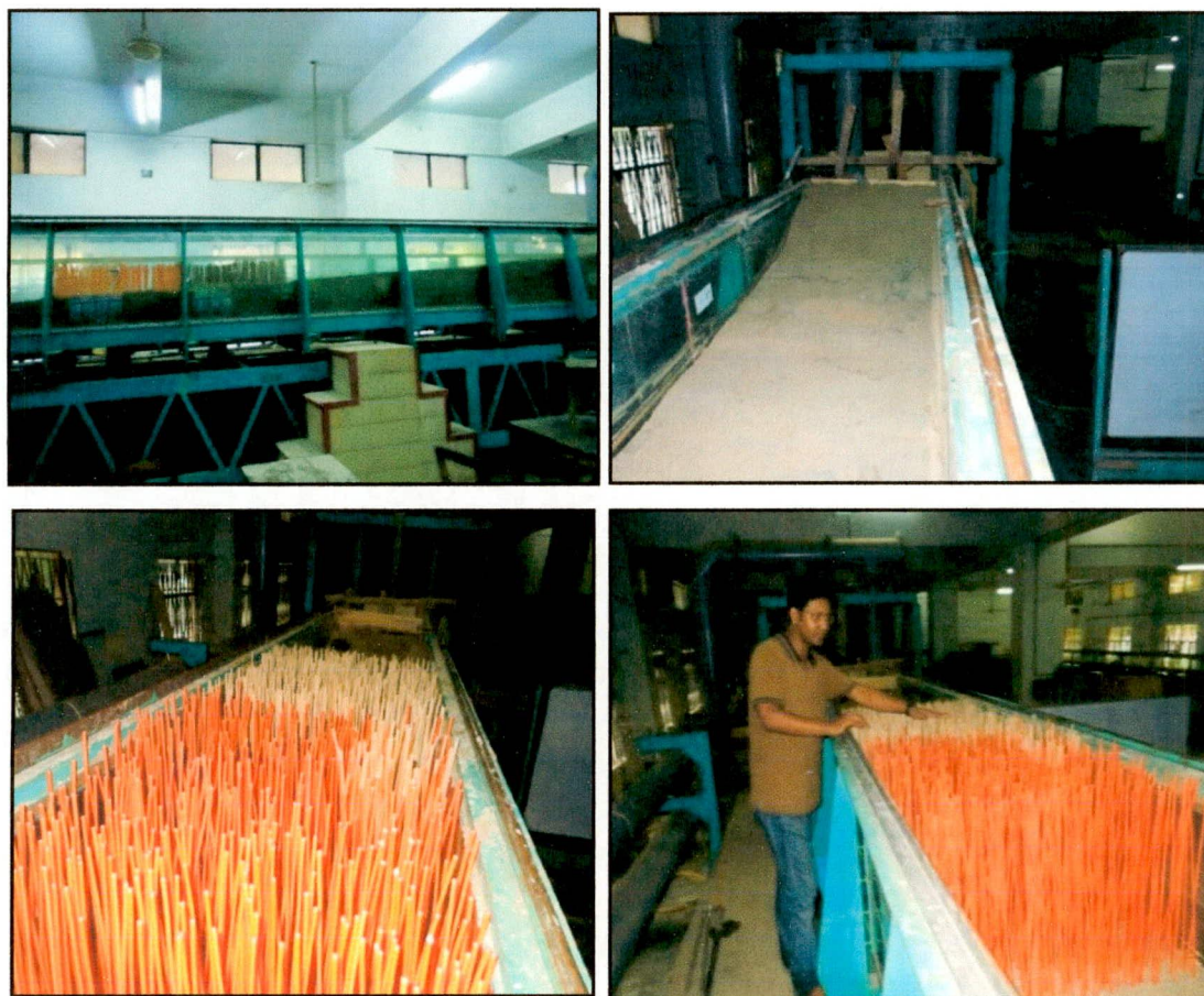
Figure: 3.7: Photographs showing preparation of experimental wave flume
